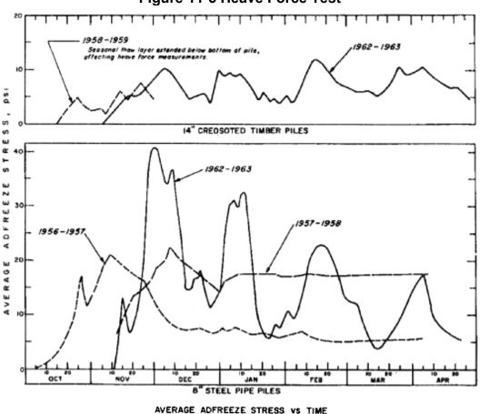
Figure 11-5 Heave Force Test
