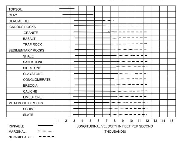
FIGURE 8-1.8 Suggested Guide for Ease of Excavation
