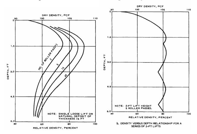
Figure 8-7.3 Sand Densification Using Vibratory Rollers
