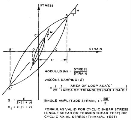
Figure 12-9 Idealized Cyclic Stress-Strain Loop for Soil
