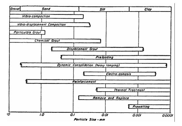
Figure 8-7.1 Applicable Grain-size Ranges for Different Stabilization Methods
