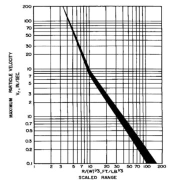
FIGURE 8-1.9 Cube Root Scaling Versus Maximum Particle Velocity
