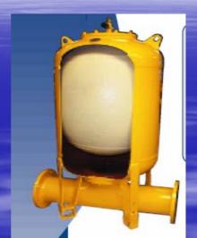
There are two types of gas accumulator used for the mitigation of surge pressures. Firstly there is a pressure vessel with a back up compressor that maintains the volume of gas in the unit to cater for pressure changes. This is shown on the following slide. The second is a pressure vessels fitted with an elastomeric bladder with gas one side and the process fluid the other.
