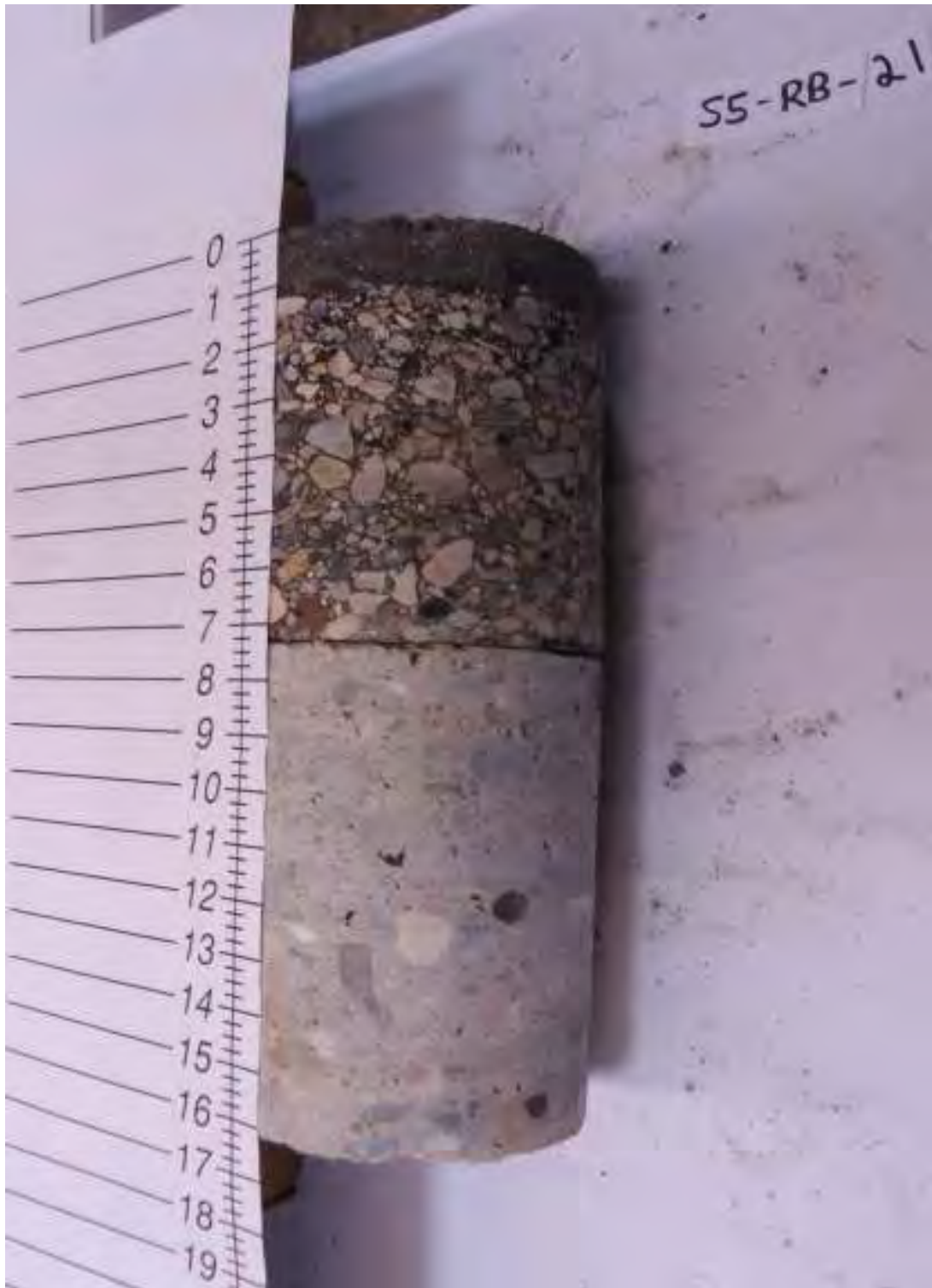
S5-RB-21: 7.25 in. Asphalt, 9 in. Concrete
