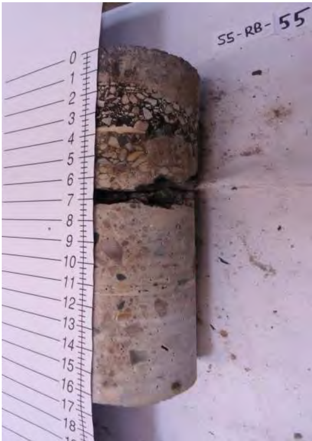
S5-RB-55: 6 in. Asphalt, 9.25 in. Concrete
