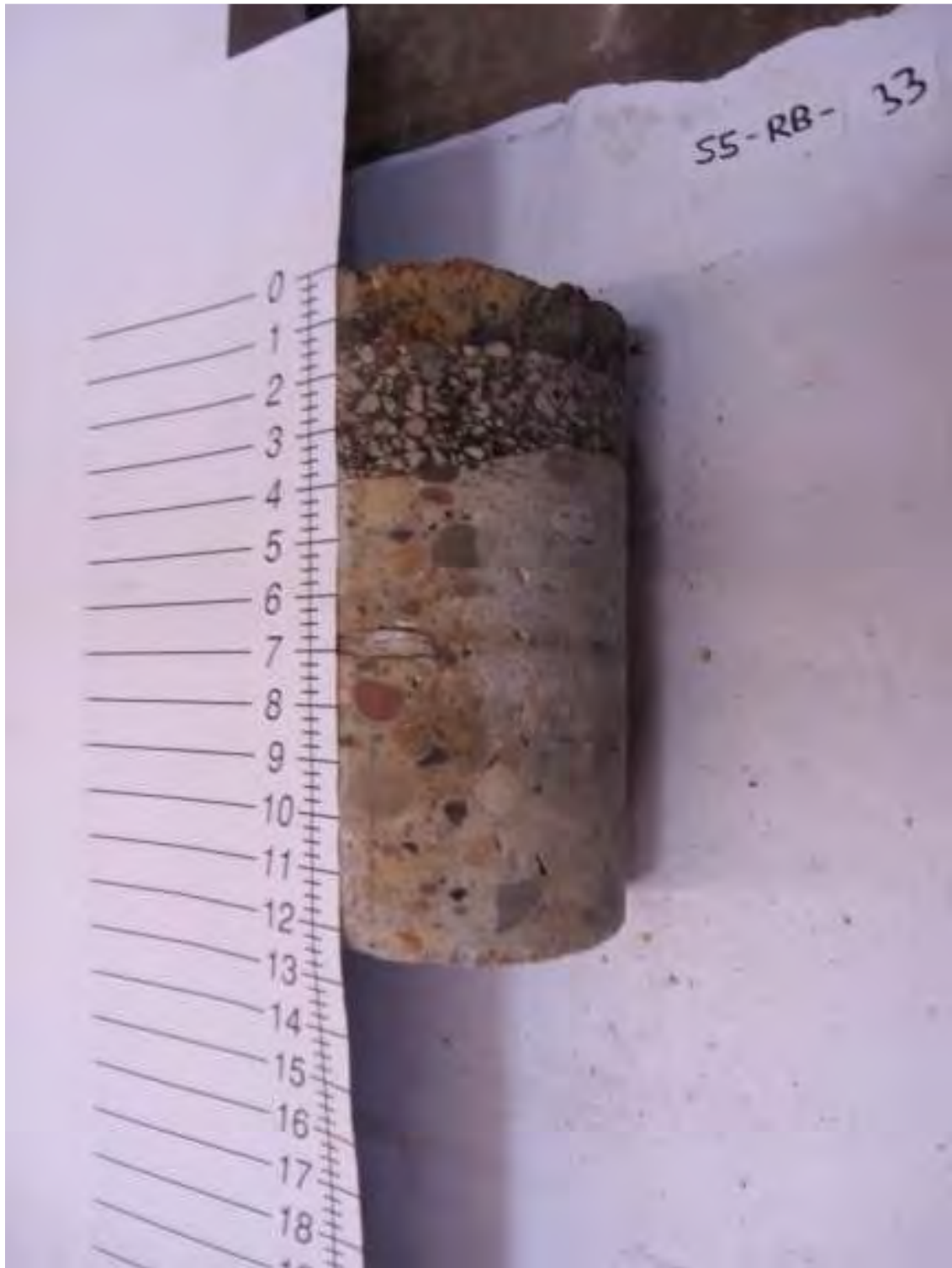
S5-RB-33: 4 in. Asphalt, 8.5 in. Concrete
