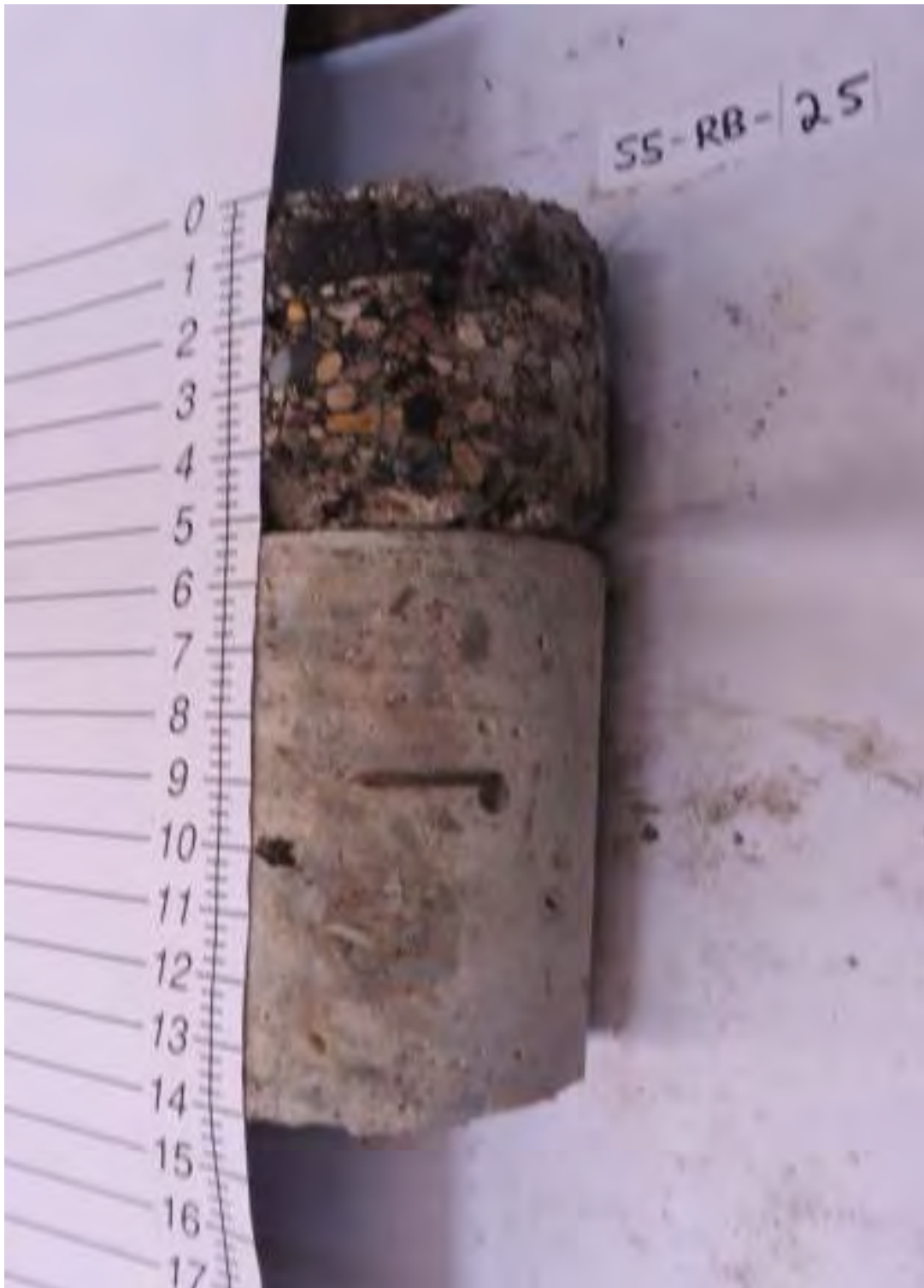
S5-RB-25: 5.25 in. Asphalt, 9 in. Concrete
