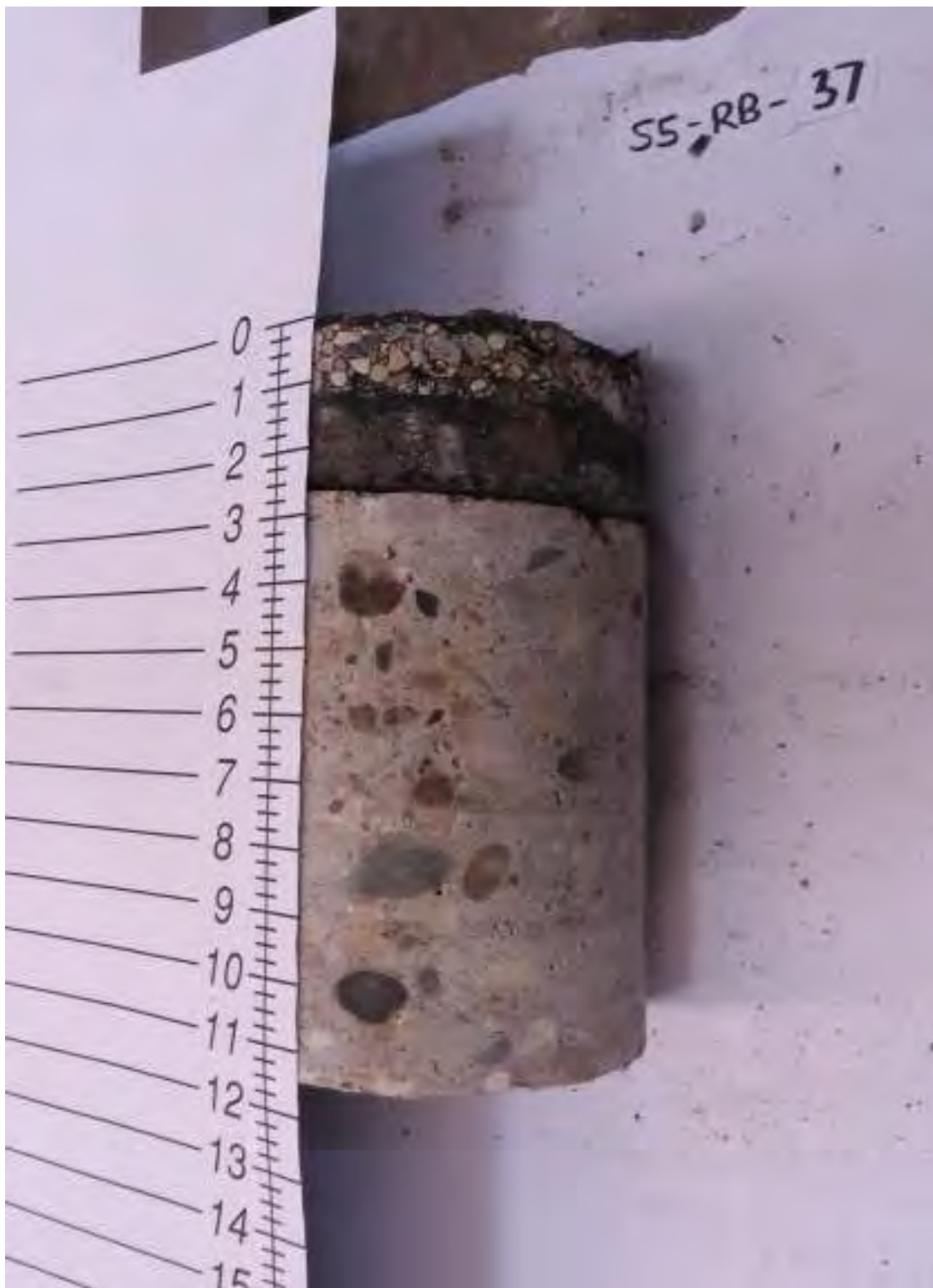
S5-RB-37: 2.75 in. Asphalt, 8.75 in. Concrete
