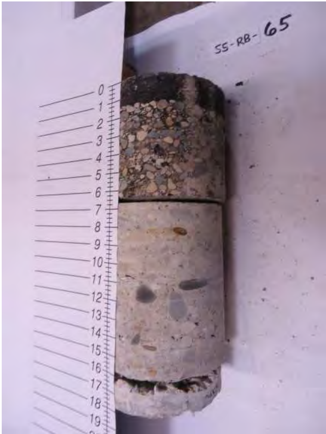
S5-RB-65: 6.5 in. Asphalt, 9.75 in. Concrete
