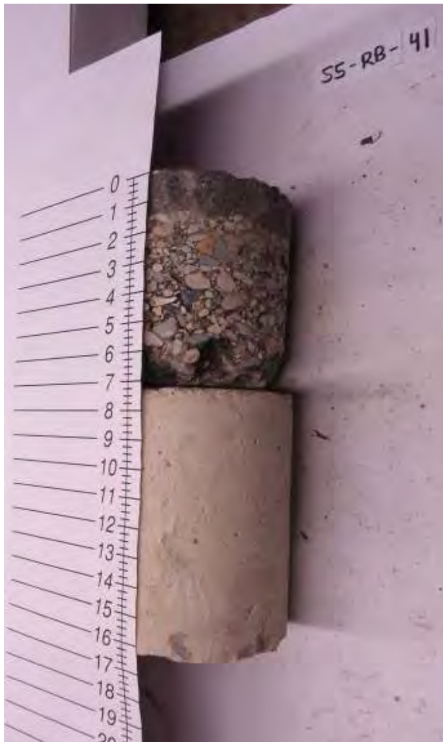
S5-RB-41: 7.25 in. Asphalt, 9 in. Concrete
