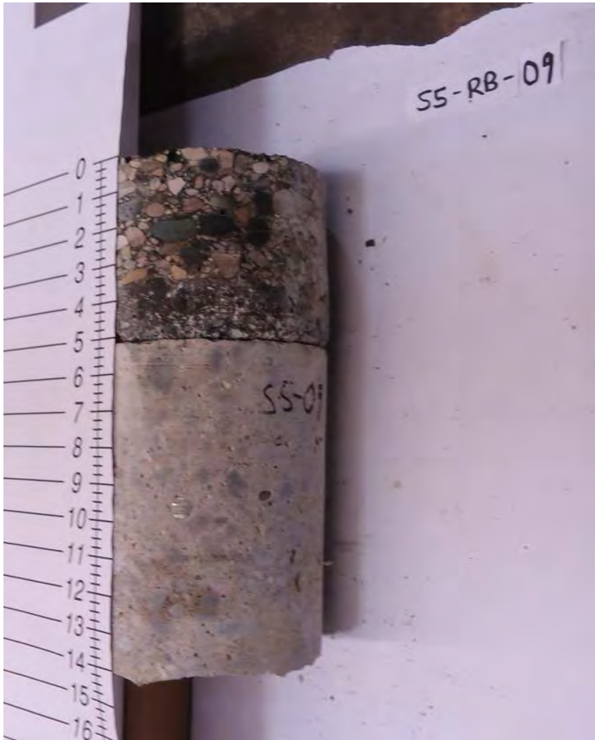
S5-RB-09: 5 in. Asphalt, 9.25 in. Concrete
