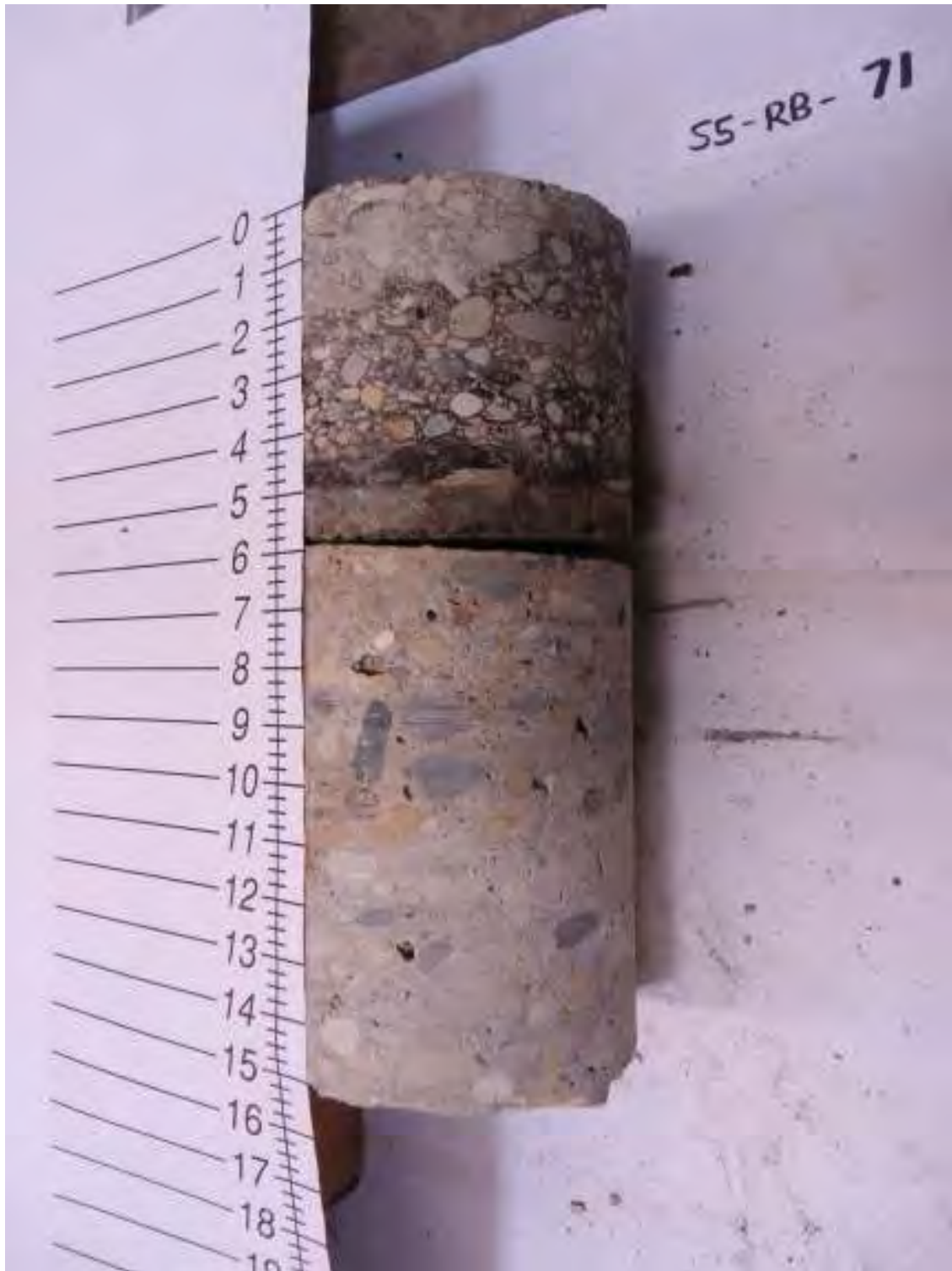
S5-RB-71: 5.75 in. Asphalt, 9.25 in. Concrete
