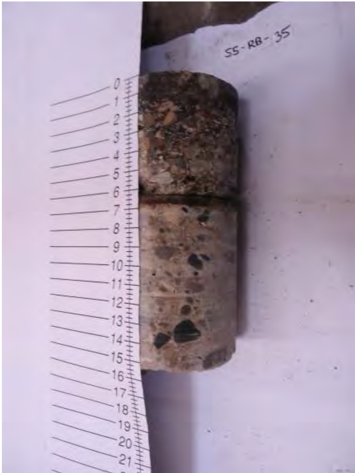
S5-RB-35: 6.25 in. Asphalt, 9.25 in. Concrete
