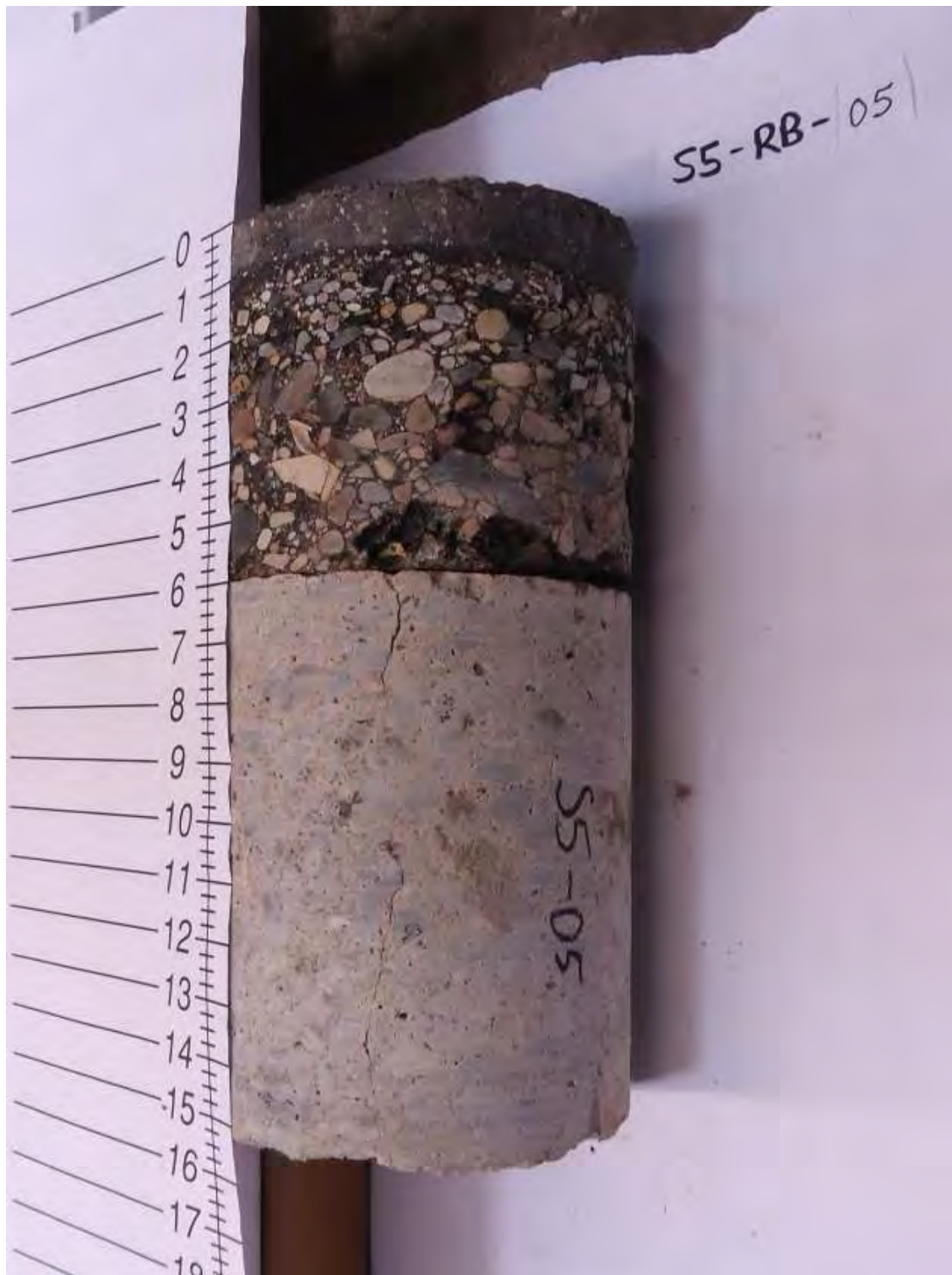
S5-RB-05: 6 in. Asphalt, 9.25 in. Concrete
