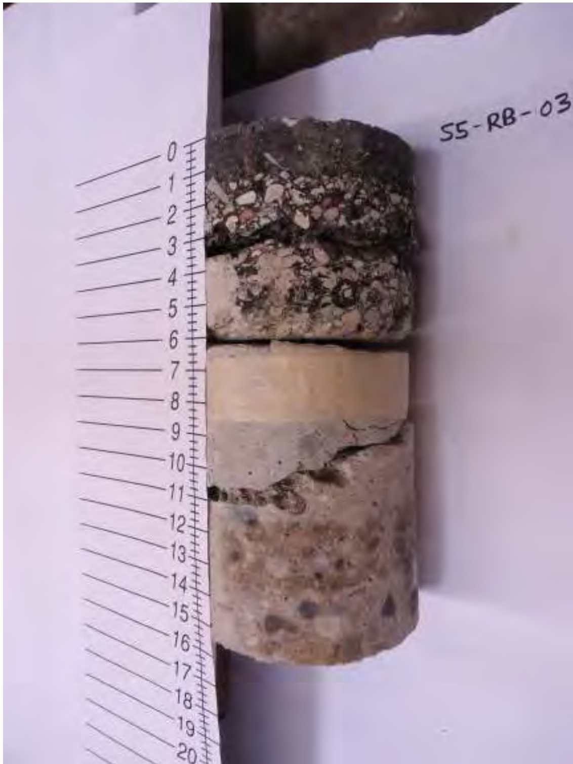
S5-RB-03: 6.25 in. Asphalt, 9.25 in. Concrete
