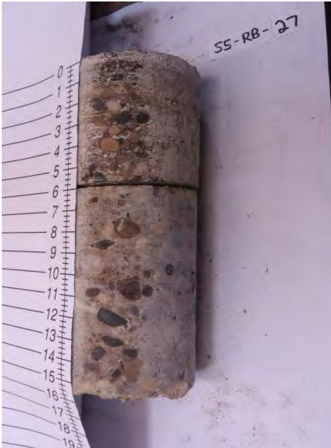
S5-RB-27: 3 in. Asphalt, 8 in. Concrete, 4 in. Concrete
