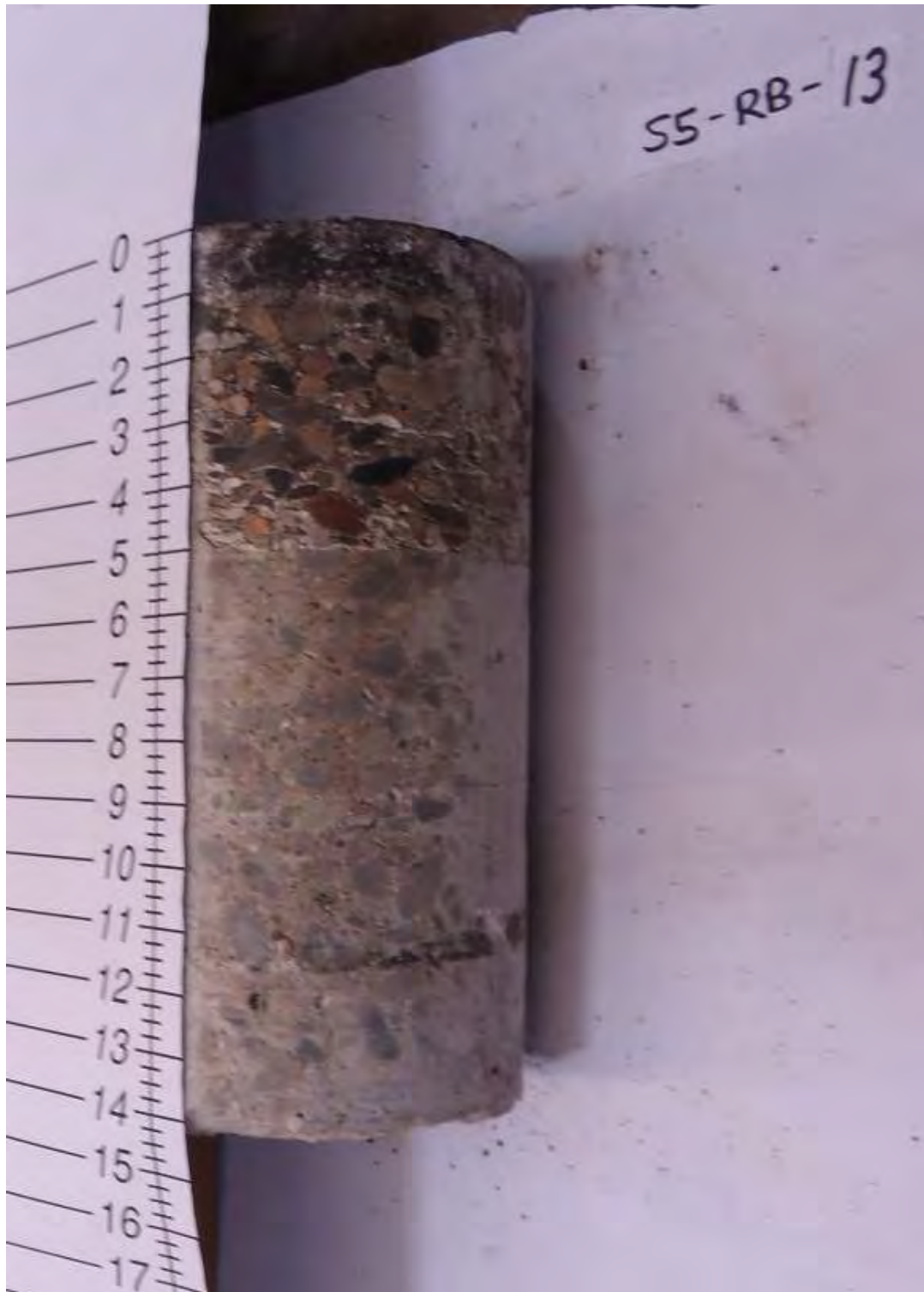
S5-RB-13: 5 in. Asphalt, 9.25 in. Concrete
