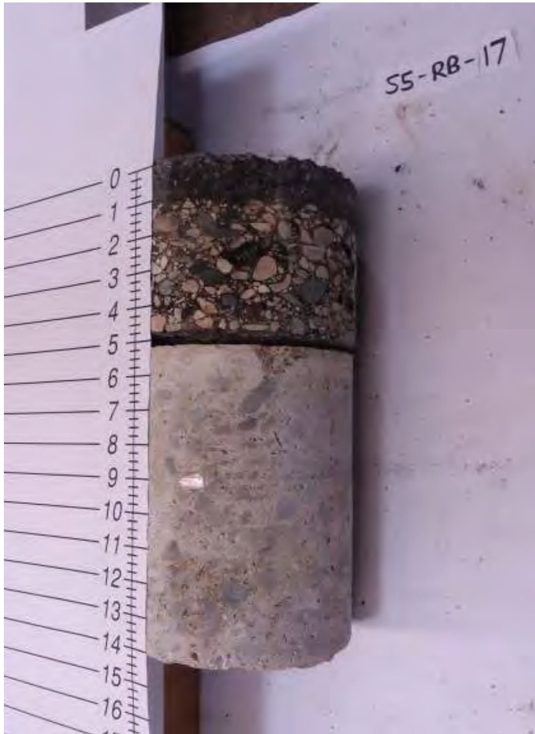
S5-RB-17: 5 in. Asphalt, 9 in. Concrete
