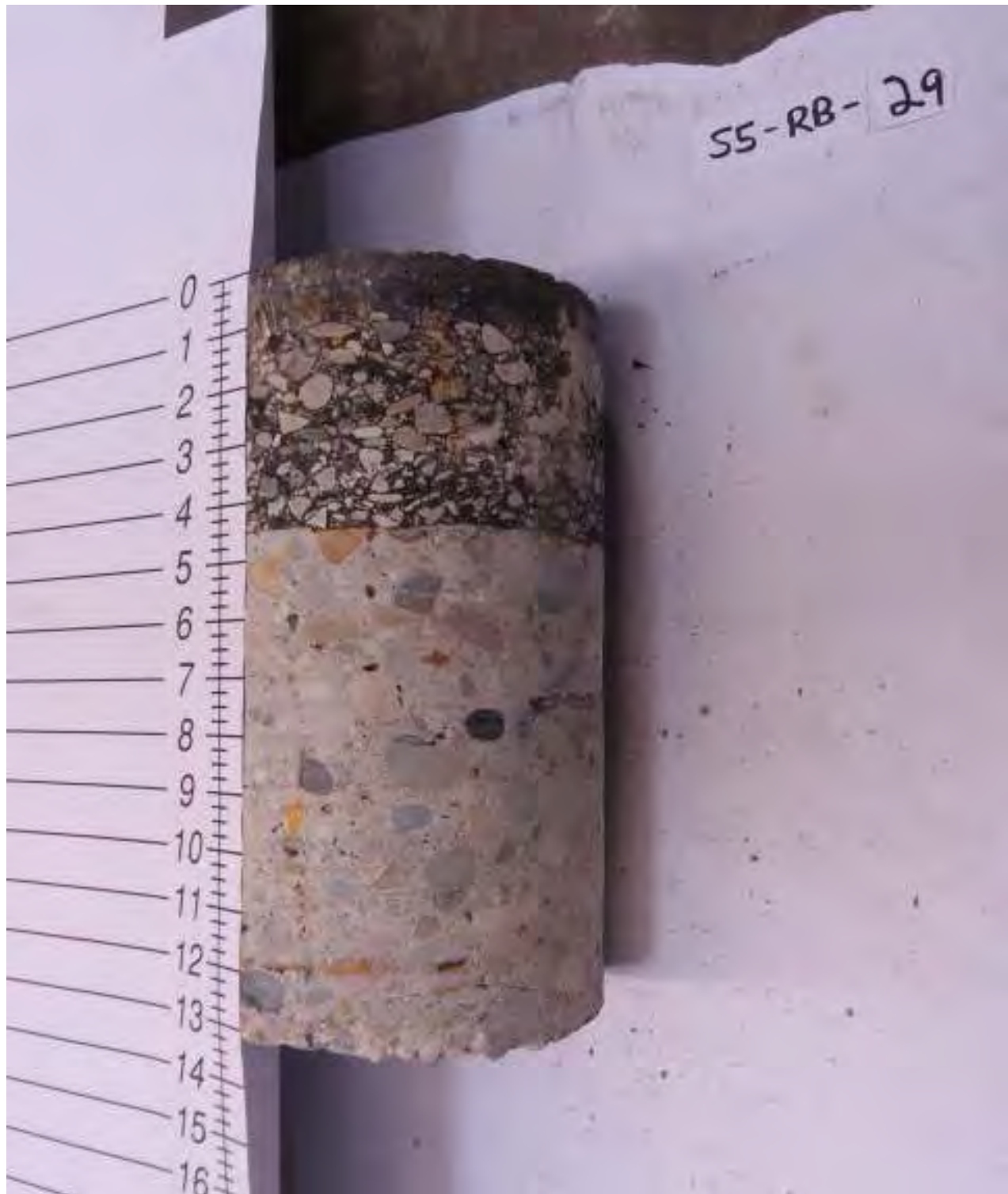
S5-RB-29: 4.5 in. Asphalt, 8.75 in. Concrete
