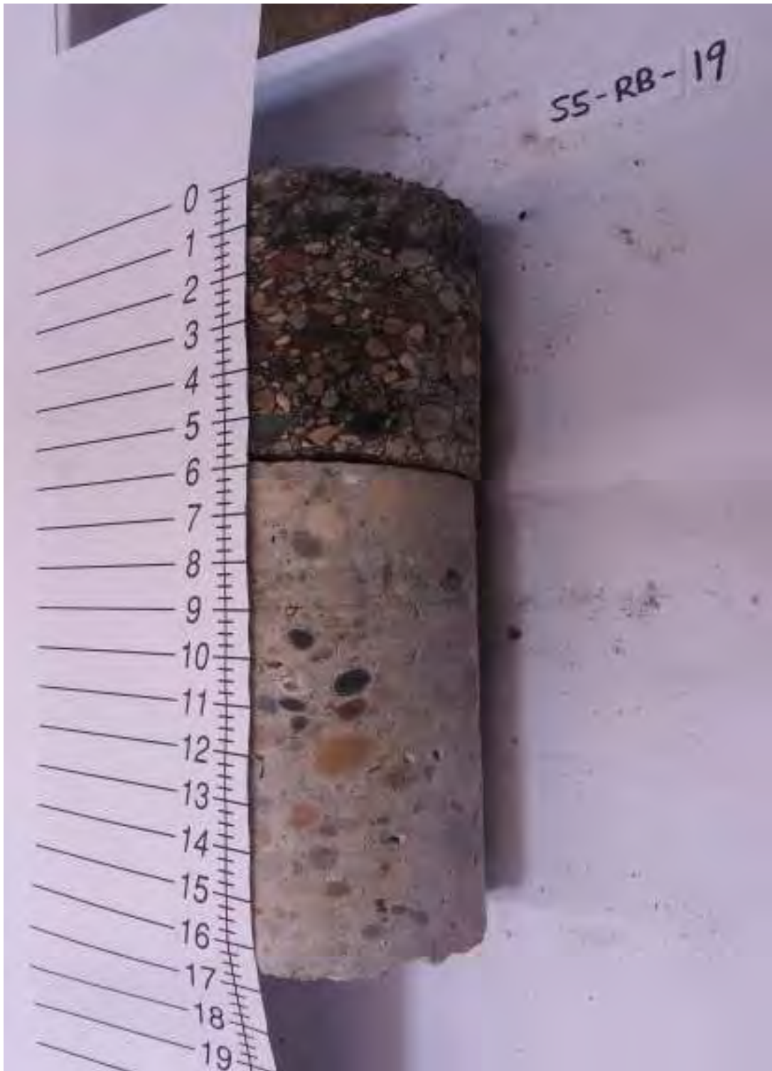
S5-RB-19: 6 in. Asphalt, 10.5 in. Concrete
