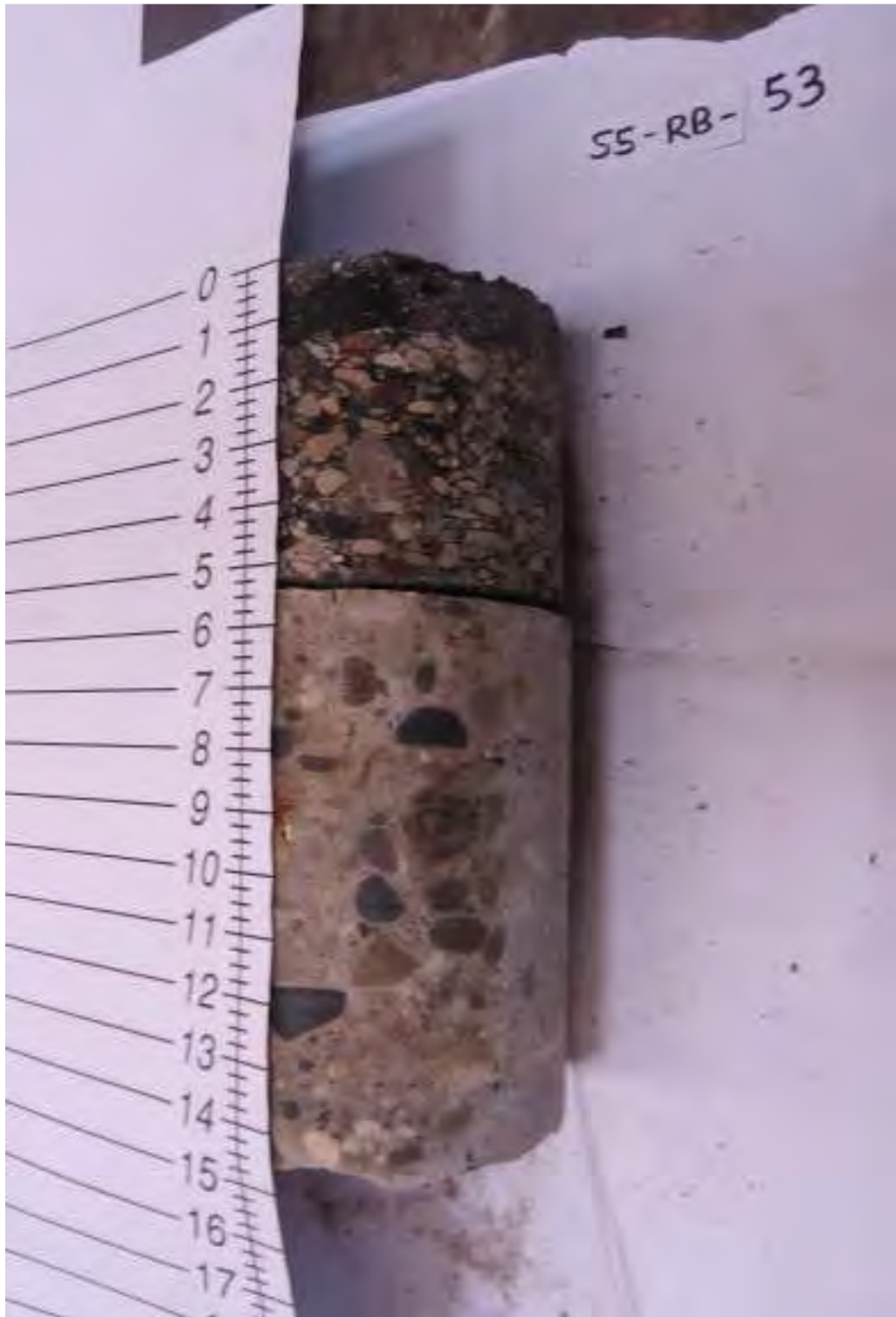
S5-RB-53: 5.25 in. Asphalt, 9.25 in. Concrete
