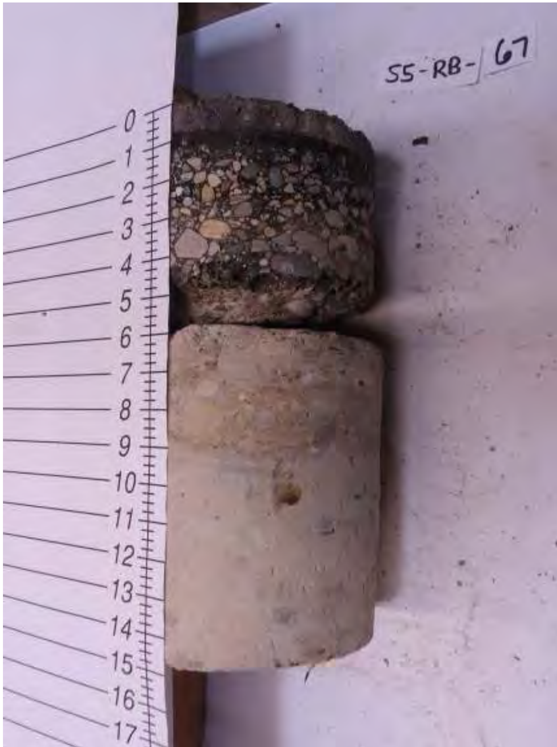
S5-RB-67: 5.75 in. Asphalt, 9 in. Concrete
