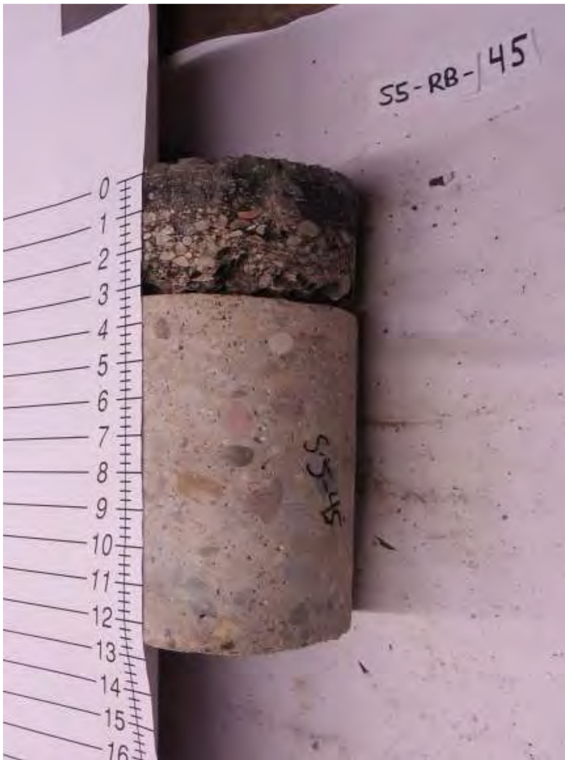
S5-RB-45: 3.25 in. Asphalt, 9.25 in. Concrete
