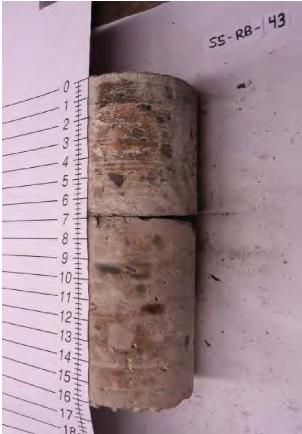
S5-RB-43: 7 in. Asphalt, 9.25 in. Concrete
