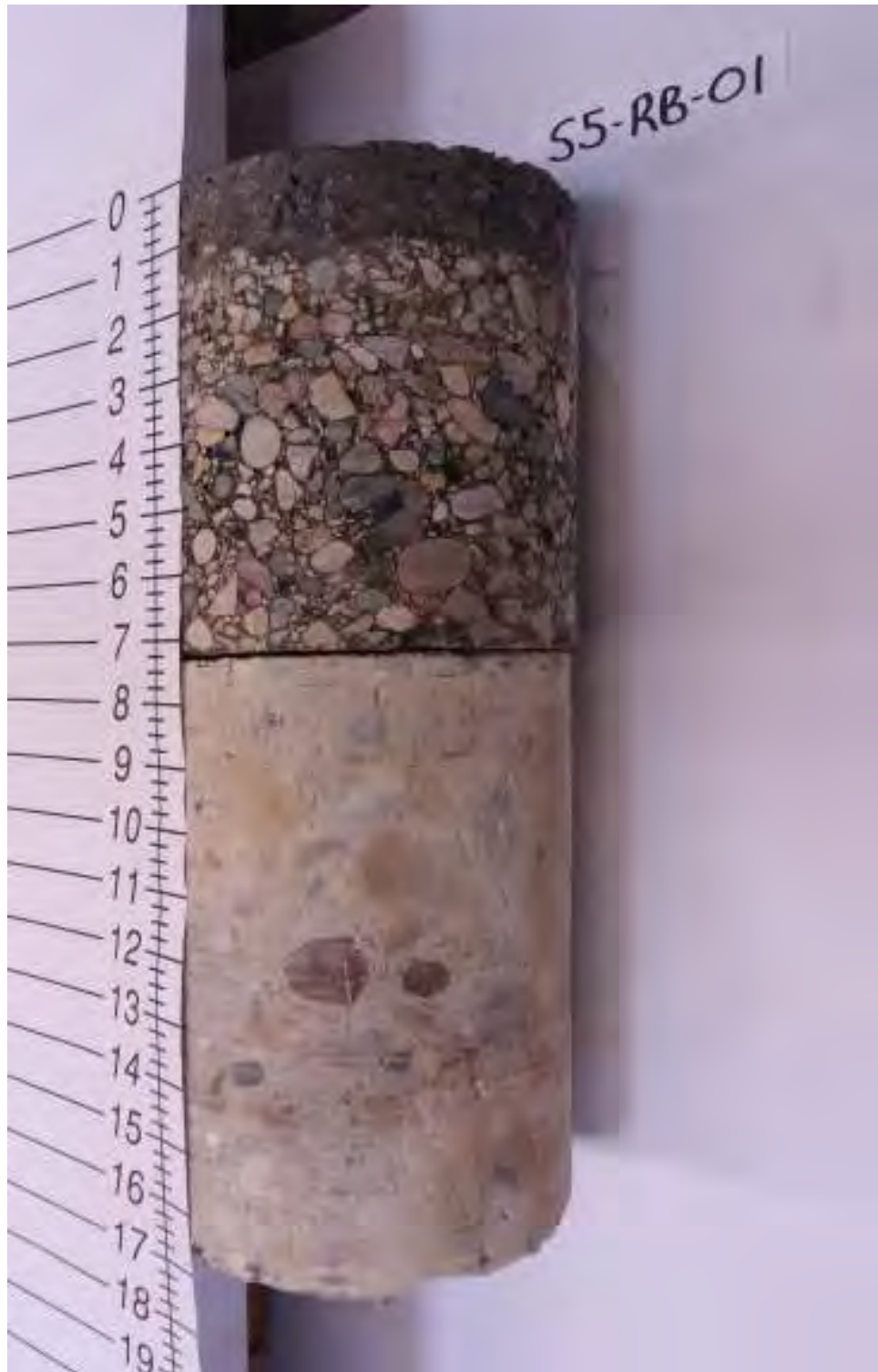
S5-RB-01: 7.25 in. Asphalt, 9.5 in. Concrete
