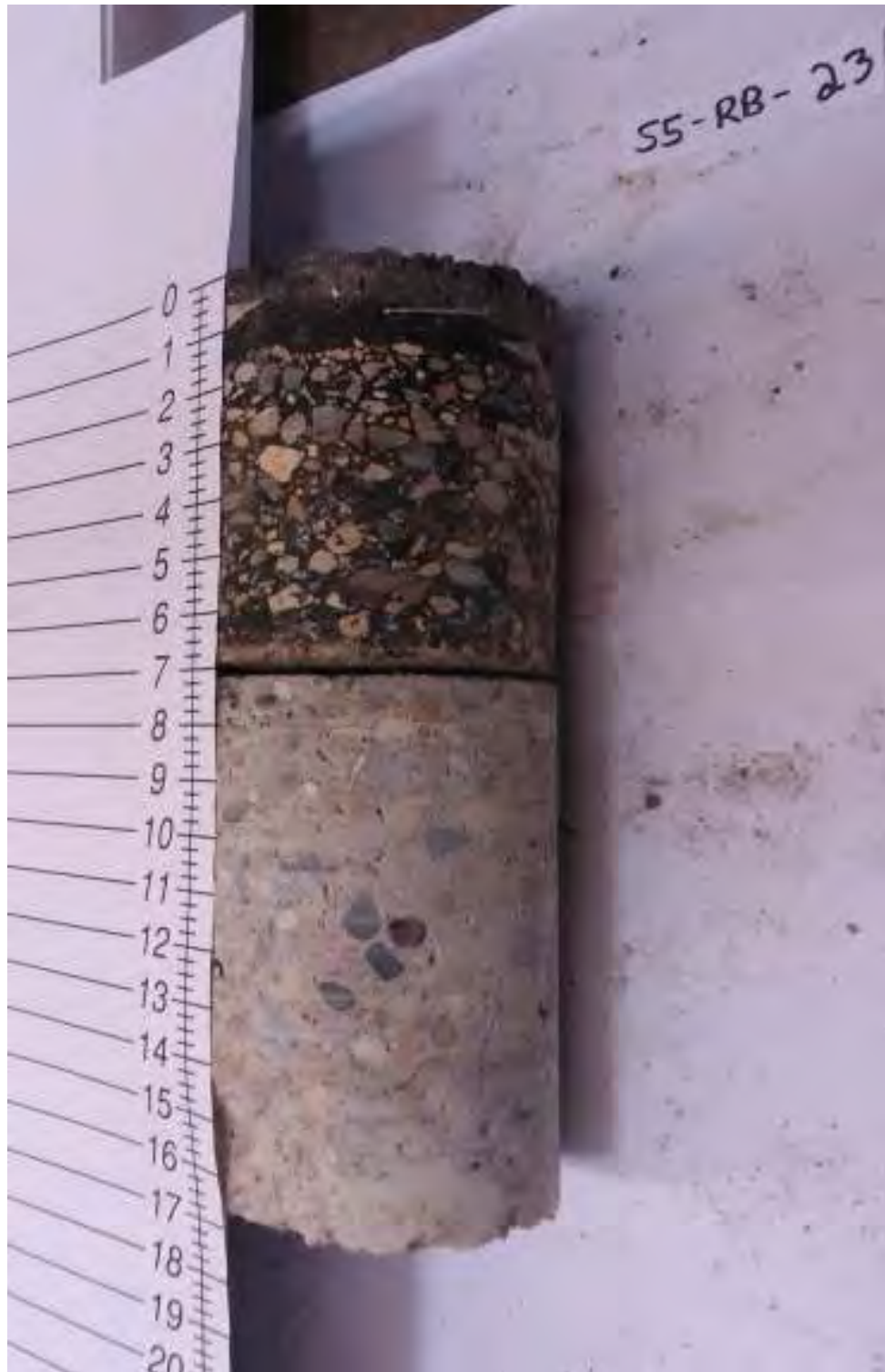
S5-RB-23: 7 in. Asphalt, 9.75 in. Concrete
