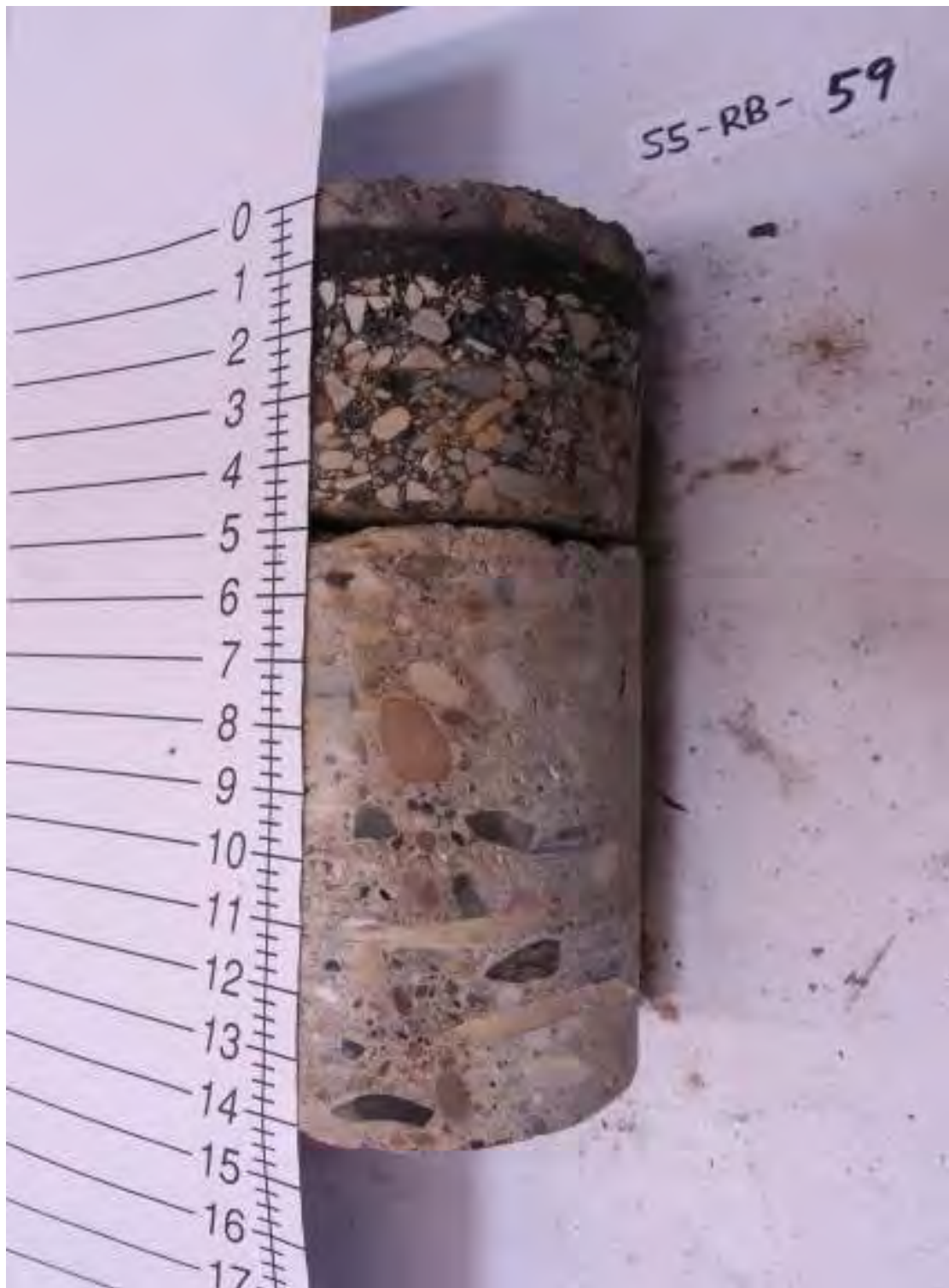
S5-RB-59: 5 in. Asphalt, 9 in. Concrete
