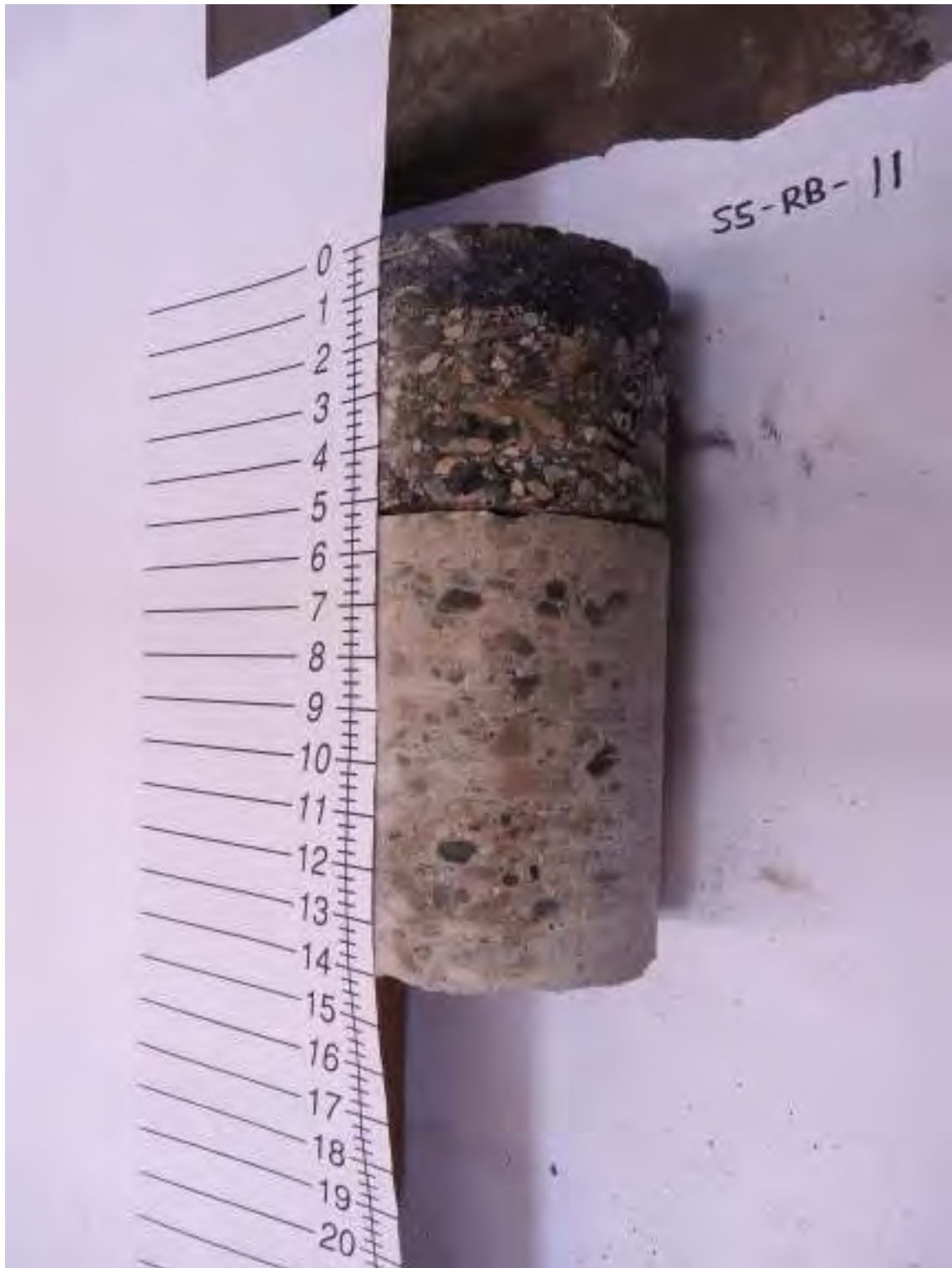
S5-RB-11: 5.25 in. Asphalt, 9 in. Concrete
