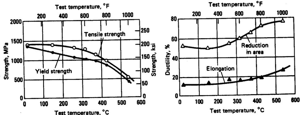
**Fig. 2** Variation in tensile properties with temperature for 4340 steel. Properties determined using specimens heat treated to a room-temperature tensile strength of 1380 MPa (200 ksi). Source: Ref 1, 3
