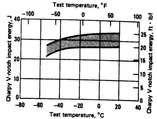
**Fig. 10** Low-temperature toughness of 8640 steel. Determined for material oil quenched and tempered to room-temperature hardness of 401 to 415 HB
