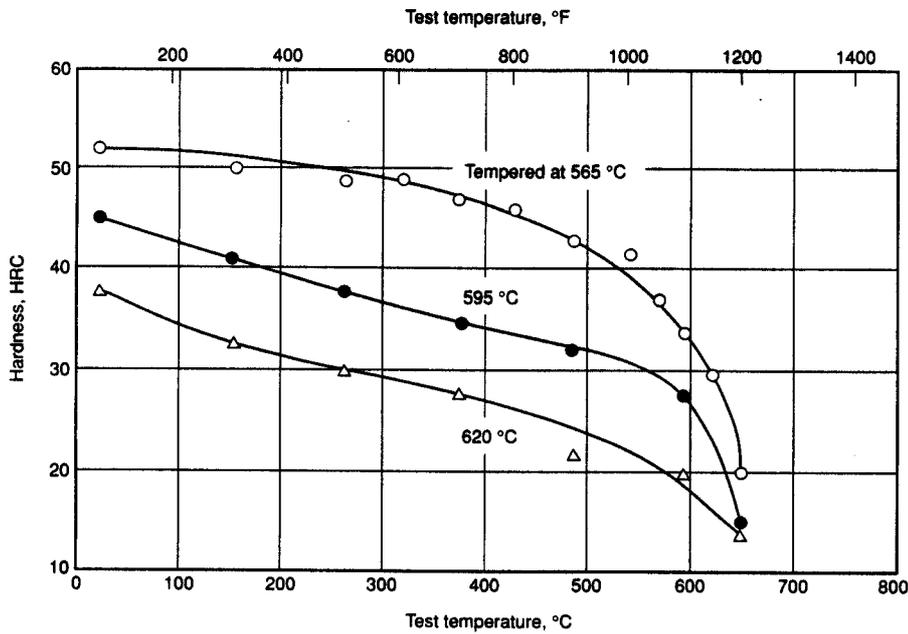
Fig. 12 Typical hot hardness of H11 mod steel. Specimens air cooled from 1010 °C (1850 °F) and double tempered, 2 + 2 h at indicated tempering temperature. Rockwell hardness converted from micro-hardness values
