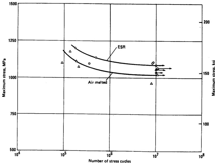
**Fig. 15** Tension-tension fatigue curves for longitudinal specimens of air-melted and electroslag-remelted heats of H13 steel. Axial fatigue tests performed in an Ivy machine at a frequency of 60 Hz; the alternating stress was 67% of the mean stress for all tests ( $R = 0.2$ ). Arrows signify tests terminated without any sign of fatigue cracking.
