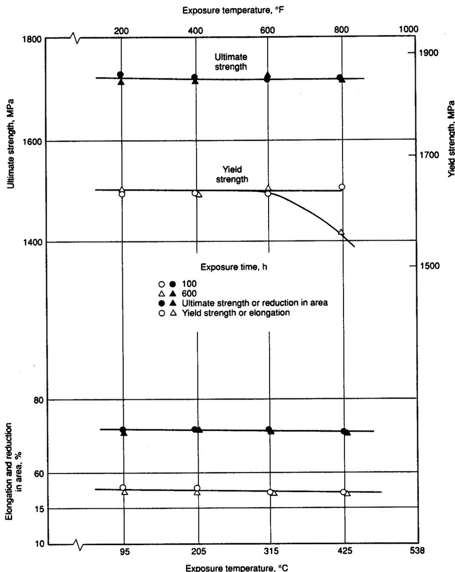
**Fig. 19** Effect of exposure to elevated temperature on room-temperature tensile properties of AF1410 steel (VIM/VAR plate 30 mm, or 1¼ in., thick). Heat treatment: Heat at 900 °C (1650 °F) for ½ h and water quench, heat at 815 °C (1500 °F) for ½ h and water quench, and then heat at 510 °C (950 °F) for 5 h and air cool. Source: Ref 1
