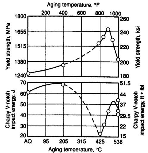
**Fig. 17** Effect of aging temperature on impact energy (bottom) and yield strength (top) of AF1410 steel (VIM/VAR plate 15 mm, or 5/8 in., thick). Heat treatments: Heat at 900 °C (1650 °F) for 1/2 h and water quench; heat at 815 °C (1500 °F) for 1/2 h and water quench; age for 5 h at indicated temperatures and air cool. AQ, as quenched. Source: Ref 1
