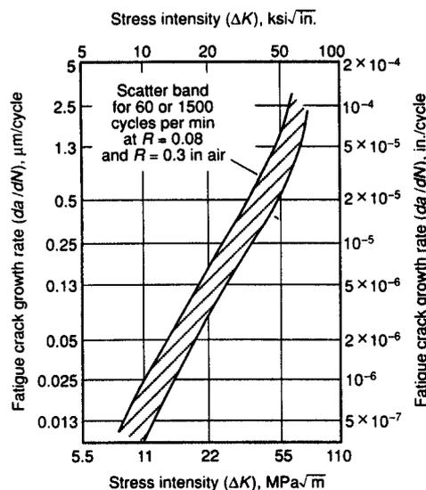
**Fig. 21** Fatigue crack growth rate at two frequencies and two  $R$  ratios for AF1410 steel (VIM/VAR plate 25 mm, or 1 in., thick) at room temperature in low-humidity air. Heat treatment same as in Fig. 20. Source: Ref 1
