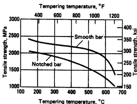
**Fig. 8** Variation in smooth-bar and notched-bar tensile strengths with tempering temperature for D-6a steel. Specimens oil quenched from 845 °C (1550 °F) and tempered 2 h at temperature. Notched bars had a stress-concentration factor,  $K_t$ , of 4.2.
