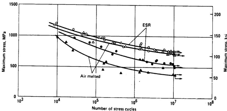
**Fig. 16** Tension-compression fatigue curves for air-melted and electroslag-remelted heats of H13 steel. Axial fatigue tests performed in an Ivy machine at a frequency of 60 Hz; the stresses were fully reversed for all tests ( $R = -1$ ). Open symbols indicate longitudinal fatigue data; filled symbols indicate transverse data. Arrows signify tests terminated without any sign of fatigue cracking. Source: Ref 10
