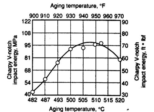
**Fig. 18** Effect of aging temperature on impact energy of AF1410 steel (VIM/VAR plate 15 mm, or 5/8 in., thick). Heat treatments: See Fig. 17.
