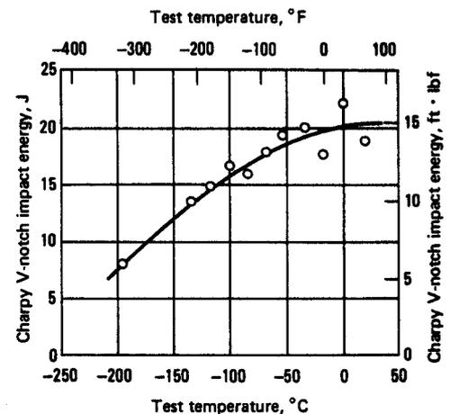
**Fig. 6** Low-temperature toughness of a D-6a steel. All specimens heat treated to a room-temperature tensile strength of 1790 to 1860 MPa (260 to 270 ksi). Each data point is the average of three tests.
