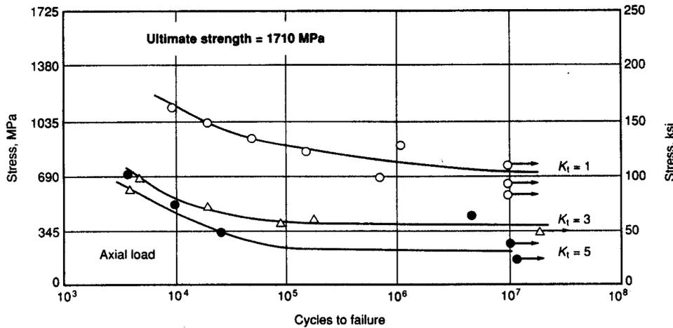
**Fig. 20** *S-N* curves at room temperature for AF1410 steel (VIM/VAR plate with 20 mm, or 3/4 in., thickness) tested in transverse direction at several stress concentrations for  $R = -1$ . Heat treatment: Heat at 900 °C (1650 °F) for 1 h and water quench, heat at 815 °C (1500 °F) for 1 h and water quench, and then heat at 510 °C (950 °F) for 5 h and air cool. Source: Ref 1
