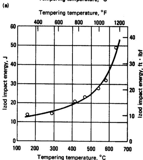
**Fig. 9** Variation in (a) hardness and (b) impact energy with tempering temperature for 6150 steel. Specimens oil quenched from 885 °C (1625 °F) and tempered 2 h at temperature
