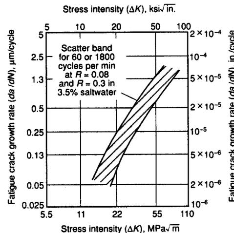
**Fig. 22** Fatigue crack growth rate at two frequencies and two  $R$  ratios for AF1410 steel (VIM/VAR plate 25 mm, or 1 in., thick) at room temperature in 3 1/2% saltwater solution. Heat treatment same as in Fig. 20. Source: Ref 1
