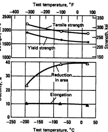
Fig. 3 Low-temperature tensile properties of 4340 steel. Properties determined for specimens quenched from 860 °C (1575 °F) and double tempered at 230 °C (450 °F). Source: Ref 1, 4
