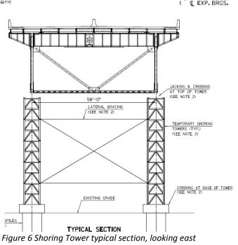
Tower construction required the relocation of aerial utilities. Additionally, the pile foundations had to be located around the underground utilities shown in Figure 5. Pile installation production rates were slower than initially anticipated due to the wet conditions and soft soils at the site, but foundation operations were completed by Friday, February 3rd.
