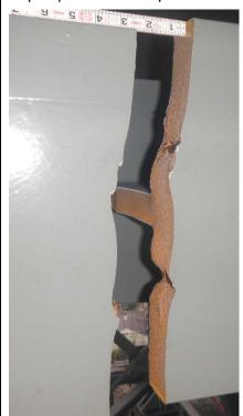
Figure 8 Close-up of north flange fracture face. (HNTB)
