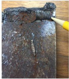
Figure 7 Sample taken from North Flange fracture surface. (HNTB)
