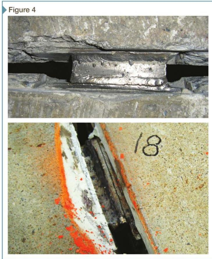
The top image is an example of fatigue failure of a flat-bar connection. At the bottom is a fatigue failure of a dowel-type connection.
