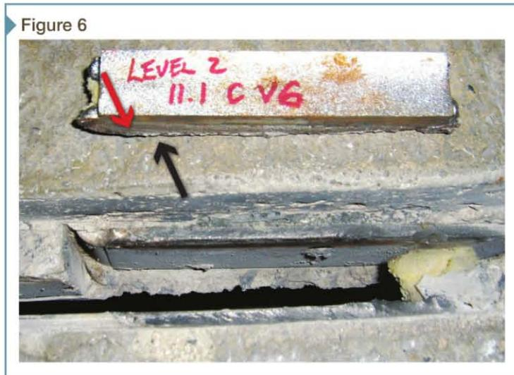
Fatigue fracture at flat erection bar (shown upside-down). Note uniform and burnished crack propagation zone and linear striations at face of weld fracture (red arrow) and abrupt fracture at face of weld (black arrow).
