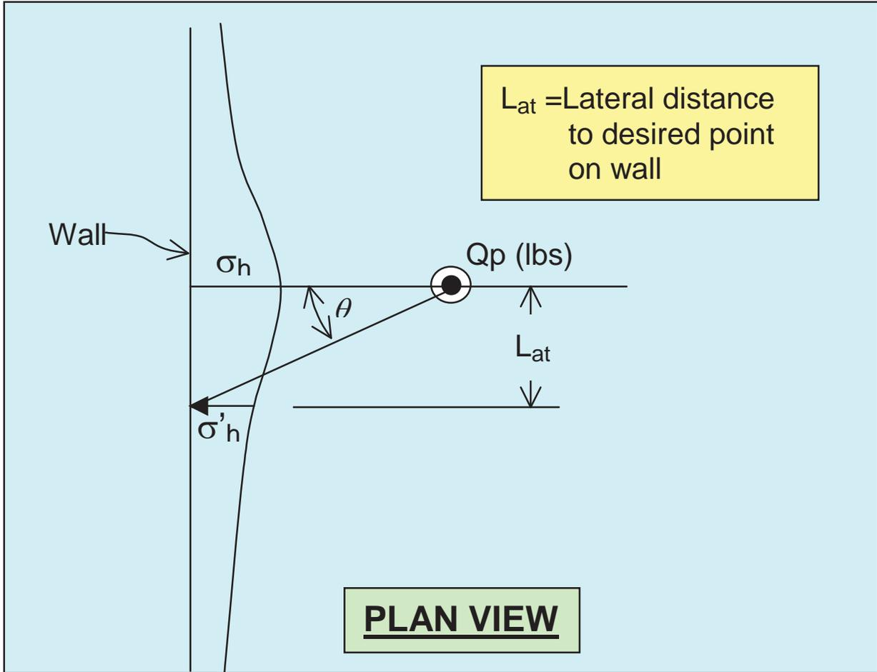
Figure 4-51. Boussinesq Type Point Load with Lateral Offset
