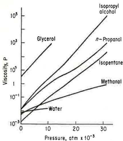
Fig. 9-16 Approximate variation of liquid viscosity with pressure at room temperature. (From Ref. 19.)
