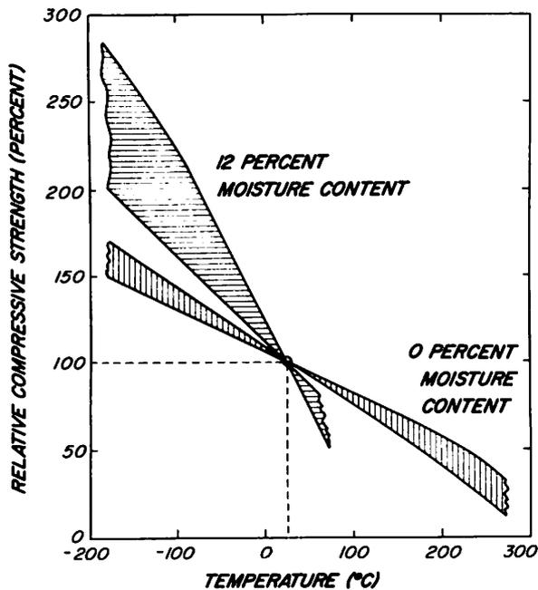
Figure 4-11—The immediate effect of temperature on compressive strength parallel to the grain at two moisture contents relative to value at 20 °C. The plot is a composite of results from several studies. Variability of reported trends is illustrated by the width of bands. (ML84 5721)
