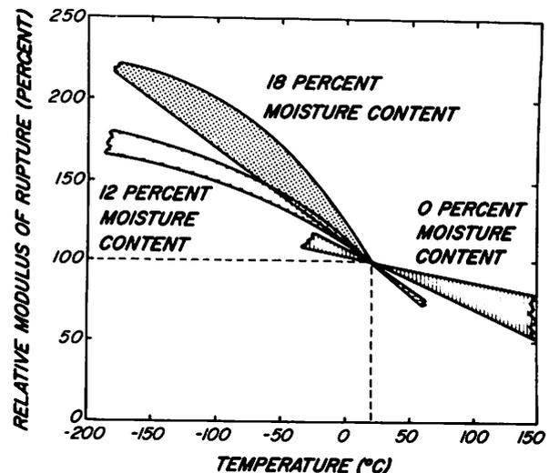
Figure 4-10—The immediate effect of temperature on modulus of rupture in bending at three moisture contents relative to value at 20 °C. The plot is a composite of results from several studies. Variability in reported trends is illustrated by the width.
