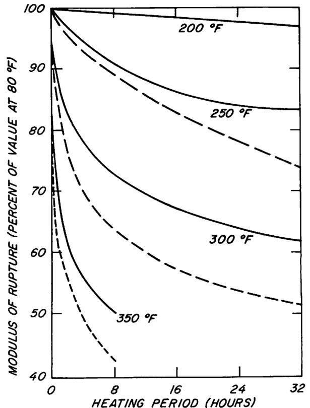
Figure 4-12—Permanent effect of heating in water (solid line) and in steam (dashed line) on the modulus of rupture. All data based on tests of Douglas-fir and Sitka spruce tested at room temperature. (M140 731)
