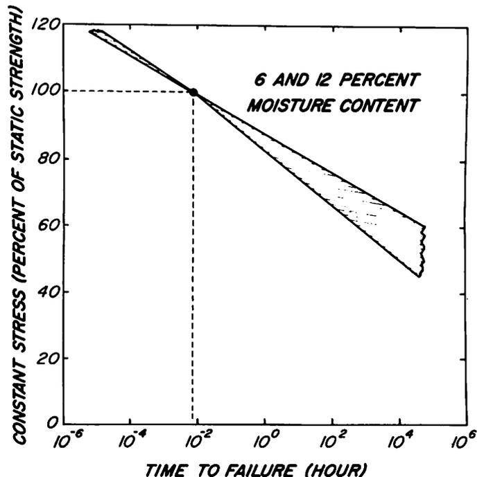
Figure 4-18—Relationship between stress due to constant load and time to failure for small clear wood specimens, based on 28 seconds' duration at 100 percent stress level. The figure is a composite of trends from several studies, mostly dealing with bending but with some on compression parallel to the grain and bending perpendicular to the grain. Variability in reported trends is indicated by the width of band.
