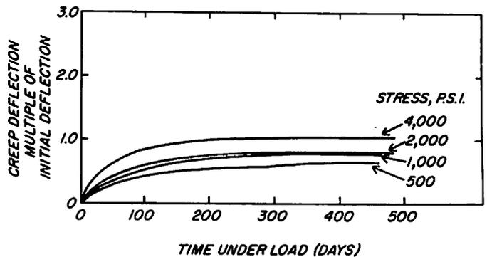
Figure 4-17—An illustration of creep as influenced by four levels of stress. (Adapted from Kingston.)
