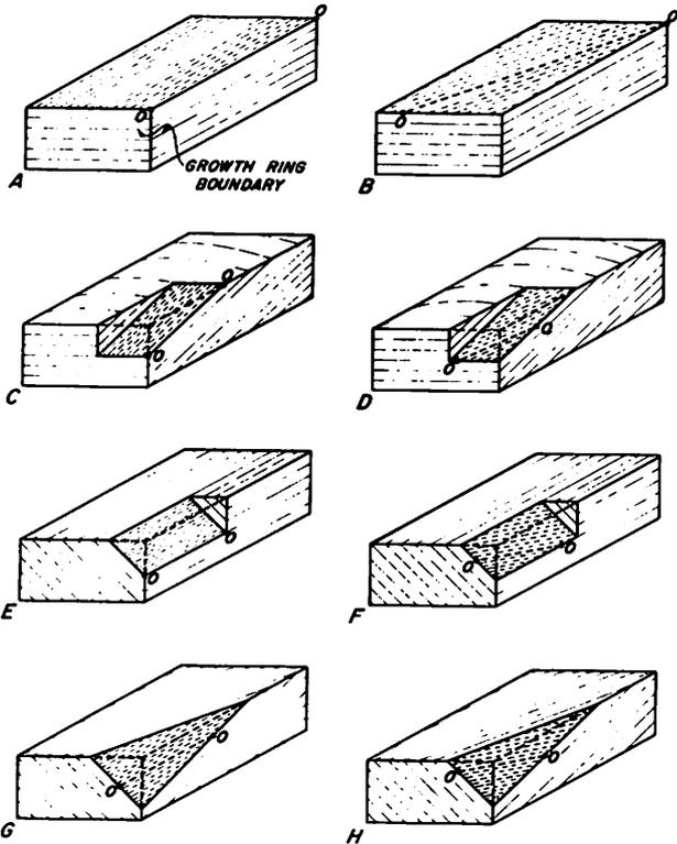
Figure 4-4—Schematic views of wood specimens containing straight grain and cross grain to illustrate the relationship of fiber orientation (0-0) to the axes of the piece. Specimens A through D have radial and tangential surfaces; E through H do not. A and E contain no cross grain. B, D, F, and H have spiral grain. C, D, G, and H have diagonal grain. (M139 385)
