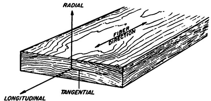
Figure 4-1—The three principal axes of wood with respect to grain direction and growth rings.
