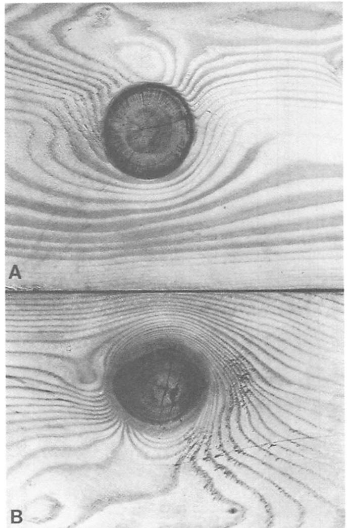
Figure 4-2—A, Encased knot. B, Intergrown knot.
