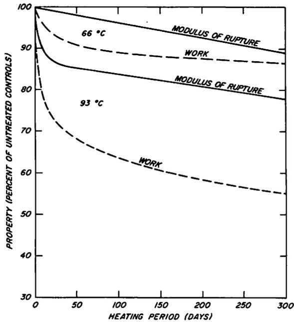
Figure 4-13—Permanent effect of heating in water on work to maximum load and on modulus of rupture. All data based on tests of Douglas-fir and Sitka spruce tested at room temperature. (M140 732)
