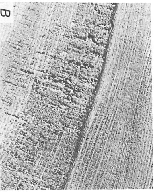
**Figure 4 – 8**—A, Compression failure is shown by the irregular lines across the grain. B, End-grain surfaces of spruce lumber show fiber breakage caused by compression failures below the dark line. (M45 594, M81 195)
