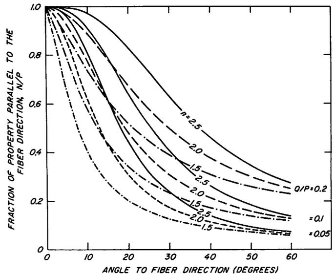
Figure 4-3—Effect of grain angle on mechanical property of clear wood according to a Hankinson-type formula.  $Q/P$  is the ratio of the mechanical property across the grain ( $Q$ ) to that parallel to the grain ( $P$ );  $n$  is an empirically determined constant.
