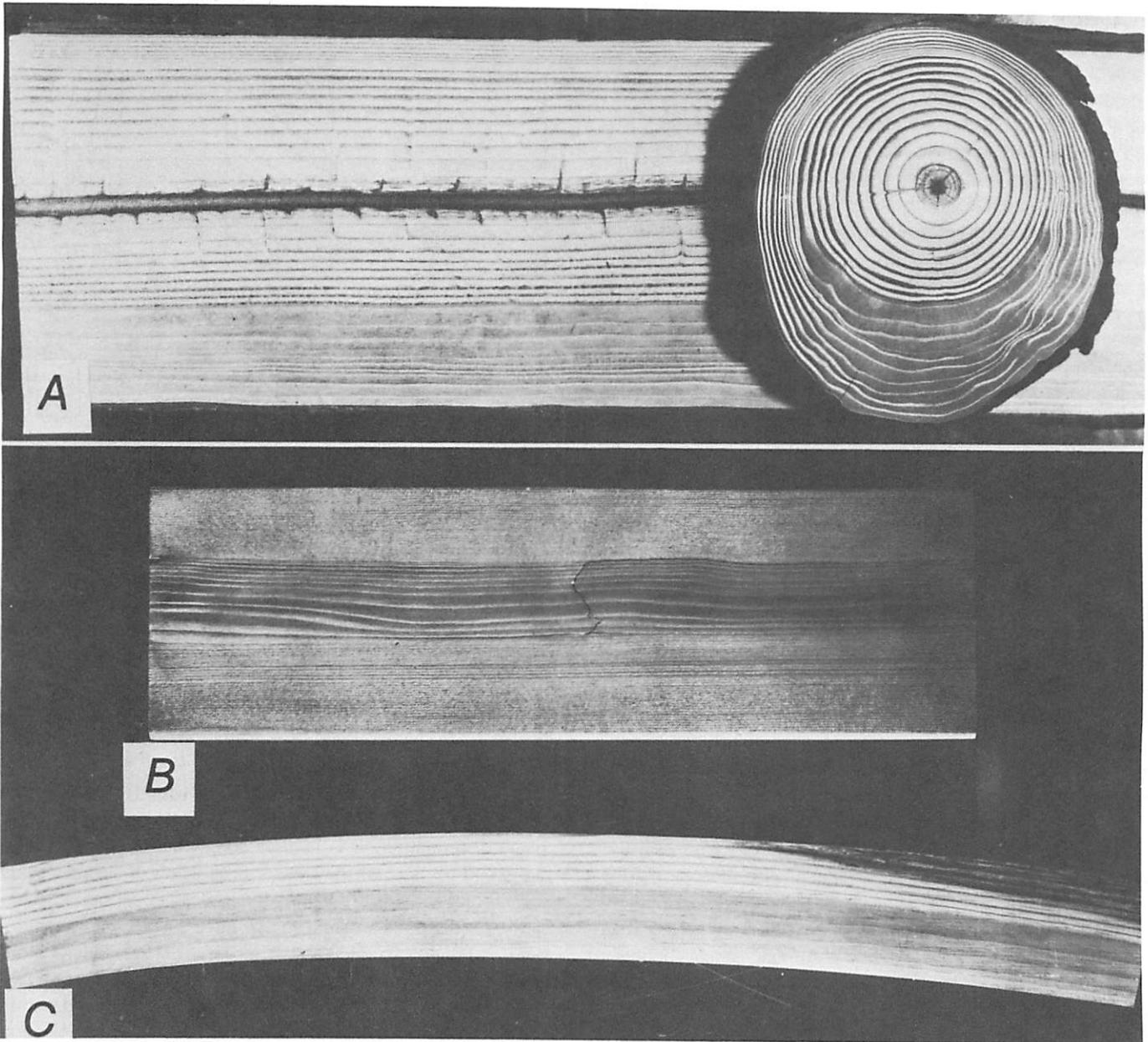
**Figure 4-6—A,** Eccentric growth about the pith in a cross section containing compression wood. The dark area in the lower third of the cross section is compression wood. **B,** Axial tension break caused by
