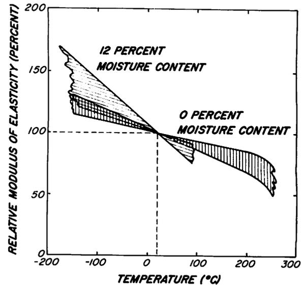
Figure 4-9—The immediate effect of temperature on modulus of elasticity parallel to the grain at two moisture contents relative to value at 20 °C. The plot is a composite of results from several studies. Variability in reported trends is illustrated by the width of bands.
