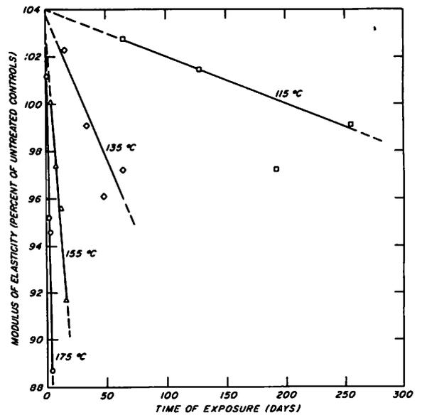
Figure 4-15—Permanent effect of oven heating at four temperatures on modulus of elasticity, based on four softwood and two hardwood species. All tests conducted at room temperature. (M140 727)
