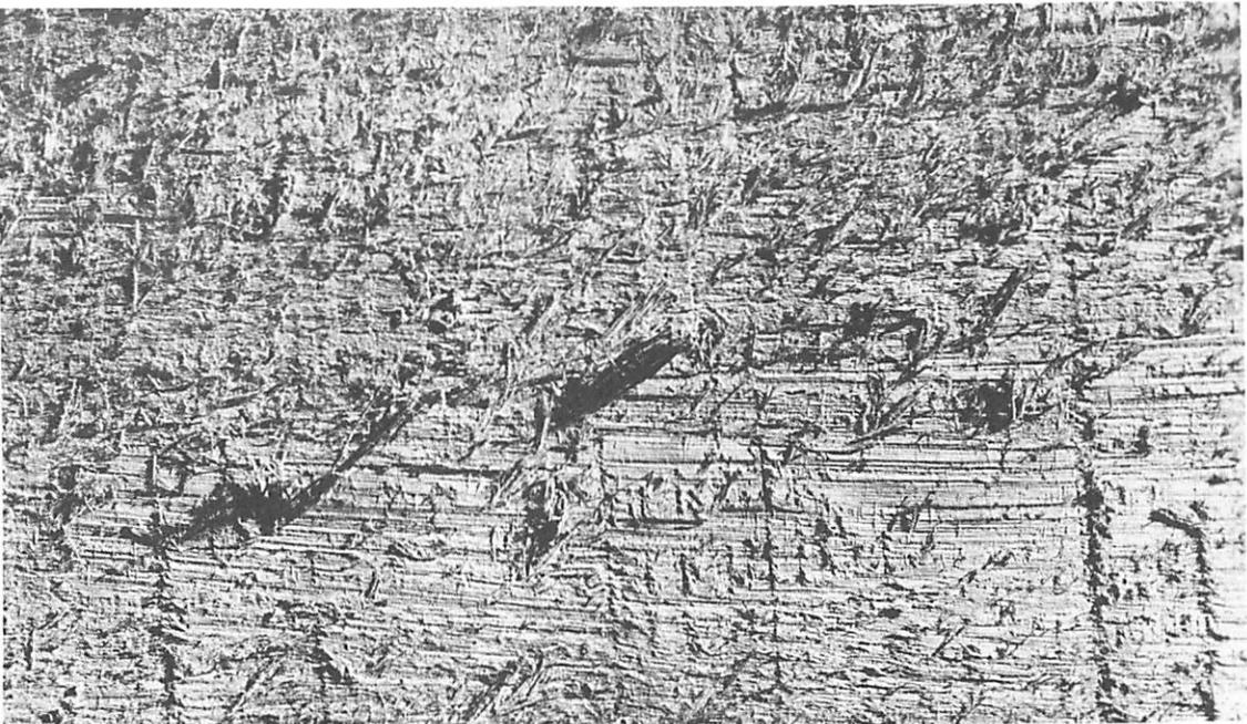
**Figure 4 – 7**—Projecting tension wood fibers on the sawn surface of a mahogany board. (M81 915)
