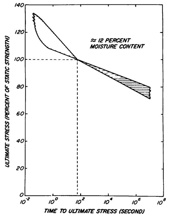
Figure 4-16—Relationship of ultimate stress at short time loading to that at 5-minute loading, based on a composite of results from rate of loading studies on bending, compression, and shear parallel to the grain. Variability in reported trends is indicated by width of band. (ML84 5722)
