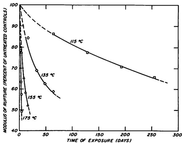
Figure 4-14—Permanent effect of oven heating at four temperatures on the modulus of rupture, based on four softwood and two hardwood species. All tests conducted at room temperature. (M140 726)
