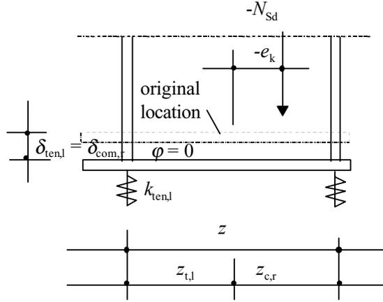
**Figure 3.3.4** Definition of  $e_k$  under zero rotation
