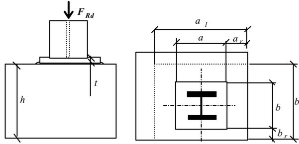
**Figure 2.1.1** Evaluation of the concrete block bearing resistance
