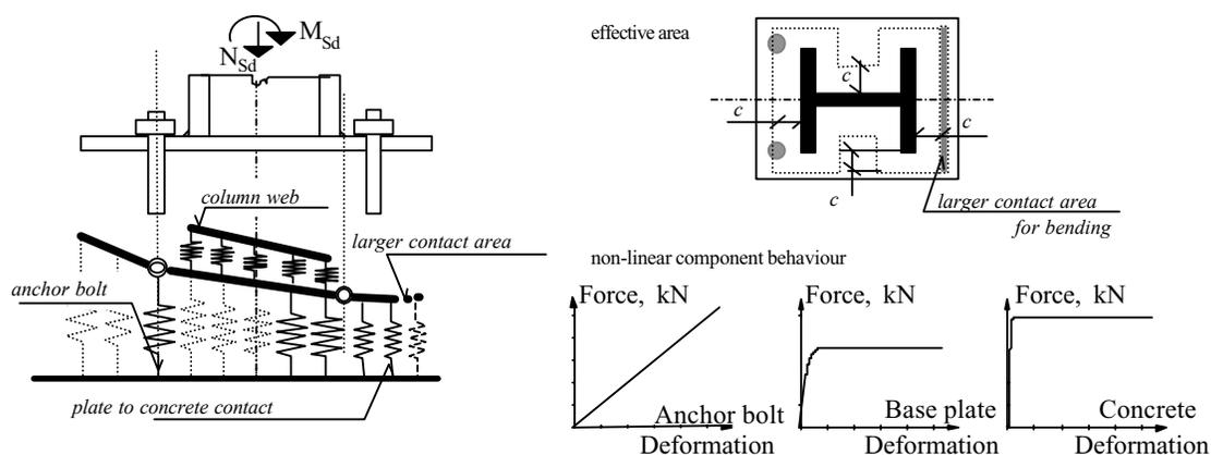
**Figure 3.2.2** Mechanical model for the assembly procedure of components according to Guisse at all, 1996
