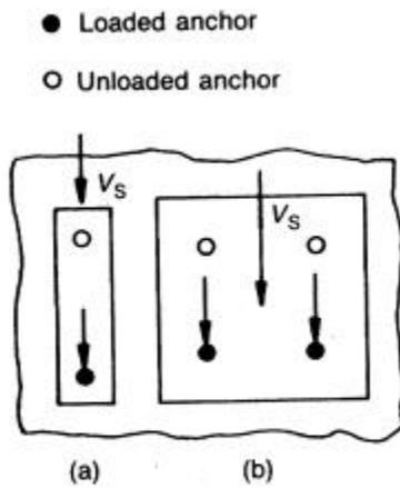
**Figure 2.4.6** Examples of load distribution if the hole clearance is large (Fig. 23 in the CEB Design Guide).
