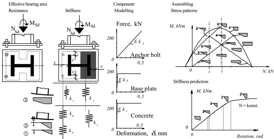
**Figure 3.2.3** The Assembly based on rectangular shape of base plate Wald, 1995, the simplification to three patterns only for high bending moments and low bending moments respectively, the bi-linear load-deformation curves of the components and the moment-normal force diagram
