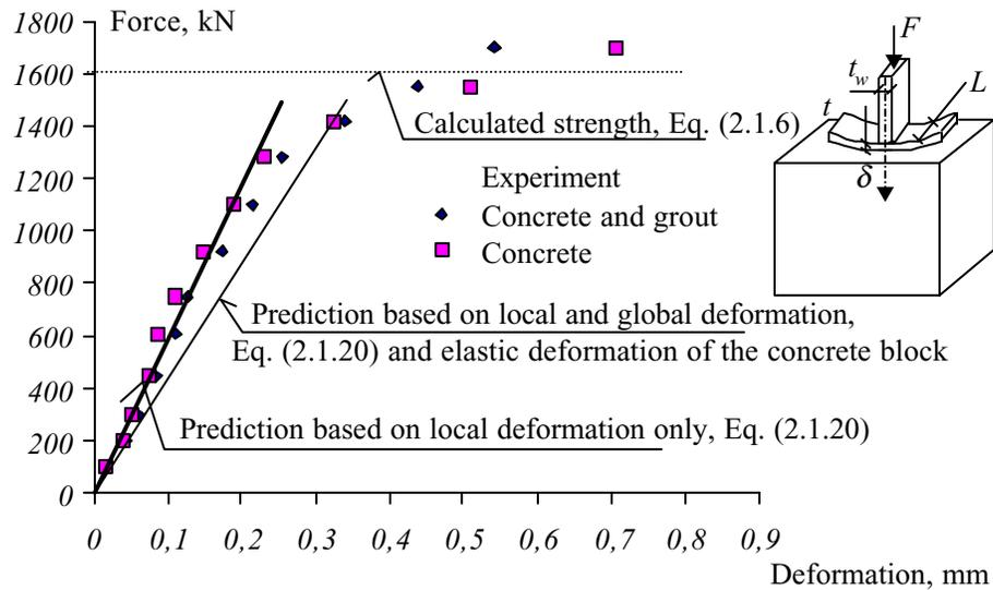
**Figure 2.1.9** Comparison of the stiffness prediction to Test 2.1, (Alma and Bijlaard, 1980), concrete block  $800 \times 400 \times 320$  mm, plate thickness  $t = 32,2$  mm, T stub length  $L = 300$  mm
