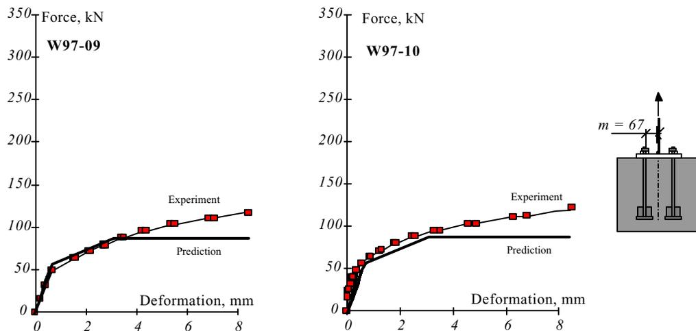
**Figure 2.3.29** Load deflection diagram for experiment W 97-09 and W 97-10. (Sokol and Wald, 1997). Bolts M24, plate 12 mm,  $m = 65$  mm,  $n = 40$  mm, concrete block 550 x 550 x 500 mm. Collapse in the concrete block (W 97-09) and no collapse reached because of very large deformations (W 97-10).
