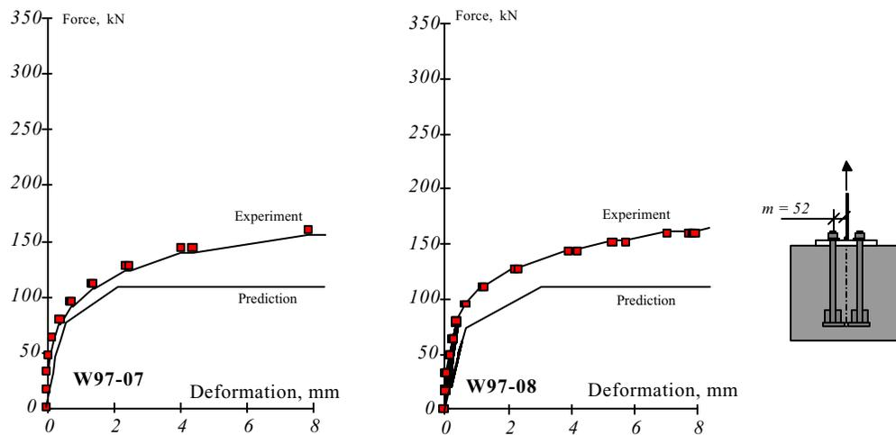
**Figure 2.3.28** Load-deflection diagrams for experiments W 97-07 and W 97-08. (Sokol and Wald, 1997). Bolts M24, plate 12 mm,  $m = 52$  mm,  $n = 40$  mm, concrete block 550 x 550 x 500 mm. Mode 1 collapse and collapse in concrete block (W 97-07) and no collapse reached because of very large deformations (W 97-08).
