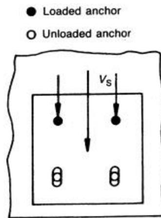
**Figure 2.4.7** Example of load distribution for an anchorage with slotted holes (Fig. 24 in the CEB Design Guide).
