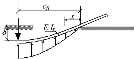
**Figure 2.1.5** A flange of a flexible T-stub
