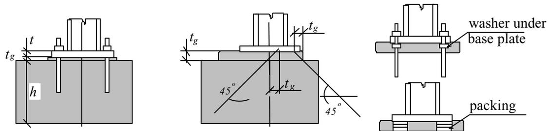
**Figure 2.1.4** The stress distribution in the grout
