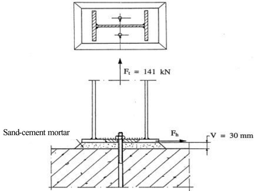
**Figure 2.4.13** Test specimen DT6.
