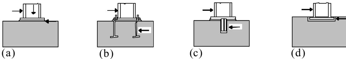
**Figure 2.4.1** Column bases loaded by horizontal shear force.
