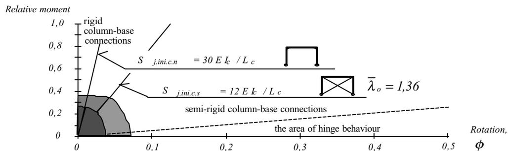
**Figure 5.7** Proposed classification system according to the initial stiffness
