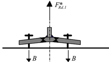
**Figure 2.3.6** Mode 1\*\* failure
