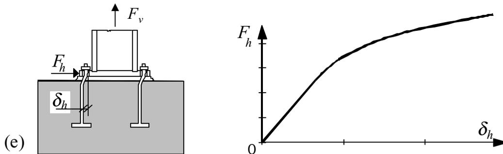
**Figure 2.4.2** Column base loaded by shear and tension.
