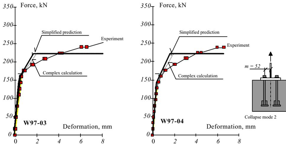
**Figure 2.3.25** Load-deflection diagrams for experiments W 97-03 and W 97-04 (Sokol and Wald, 1997). Bolts M24, plate 20 mm,  $m=52$  mm,  $n=40$  mm, concrete block  $550 \times 550 \times 500$  mm. Mode 2 collapse (breaking of bolts and plate mechanism).
