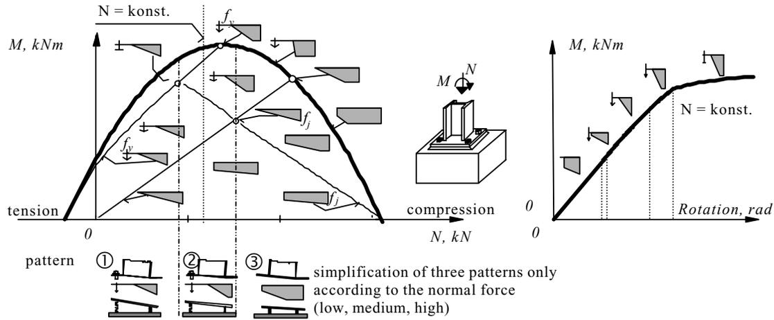
**Figure 3.2.6** Moment - normal force resistance diagram for column base introducing the internal force distribution in elastic and inelastic region,  $f_y$  is representing yielding of the tension part,  $f_j$  is bearing resistance of the concrete, see Wald, 1995
