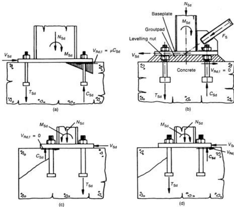
**Figure 2.4.3** Friction force due to a resulting compression reaction on the fixture. In cases (a) and (d), friction force may be considered in the design. In cases (b) and (c), friction force should not be considered in the design (Fig. 16 in the CEB Design Guide).
