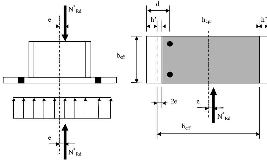
**Figure 3.2.11** Internal and external forces if no anchor bolts in tension
