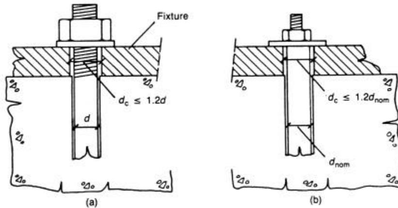
**Figure 2.4.4** Examples of anchorages with a large edge distance with a clearance hole in the fixture where all anchors will contribute to the transmission of shear forces. In case (a) the bolt is assumed to bear against fixture. In case (b) the sleeve is assumed to bear against the fixture (Fig. 20 in the CEB Design Guide).
