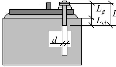
**Figure 2.3.10** Effective length of the anchor bolts
