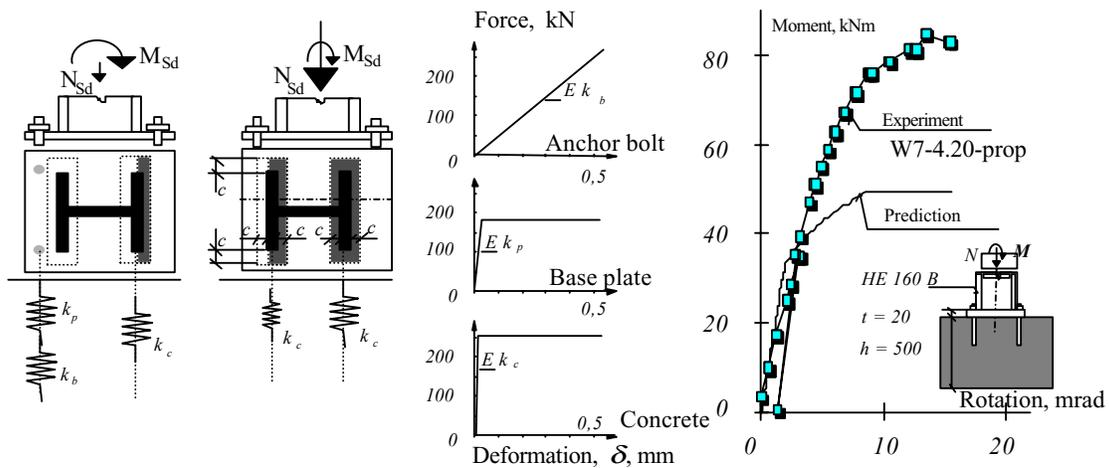
**Figure 3.2.4** The assembling with an effective area around the column flanges only Steenhuis, 1998. For high bending moments and low bending moments respectively, the bi-linear load-deformation curves of the components and the moment-rotation diagram for the joint in comparison to test no W7-4.20-prop are shown, see Wald et al, 1995
