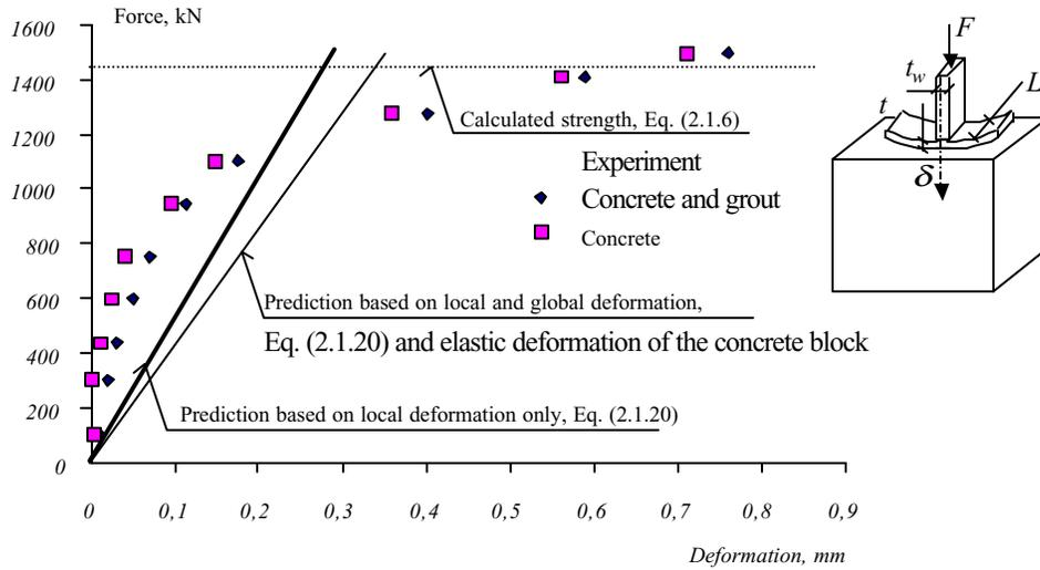
**Figure 2.1.10** Comparison of the stiffness prediction to Test 2.2, (Alma and Bijlaard, 1980), concrete block  $800 \times 400 \times 320 \text{ mm}$ , plate thickness  $t = 19 \text{ mm}$ , T stub length  $L = 300 \text{ mm}$
