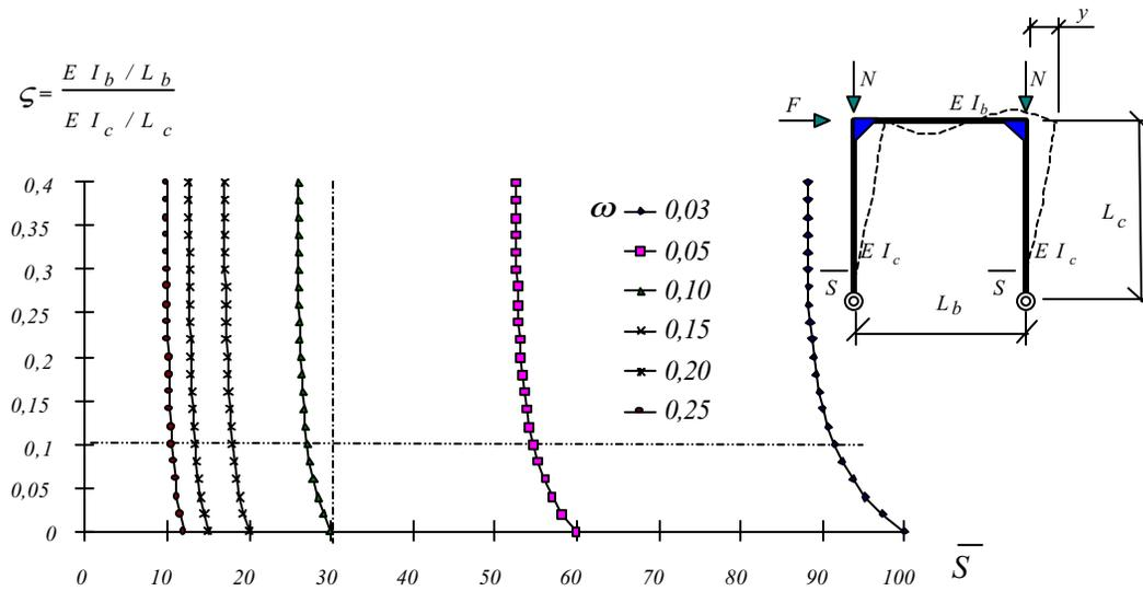
**Figure 5.6** Displacement classification criteria for column bases
