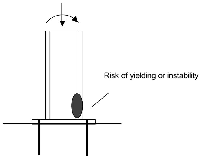
**Figure 2.2.1** Component “column flange and web in compression”
