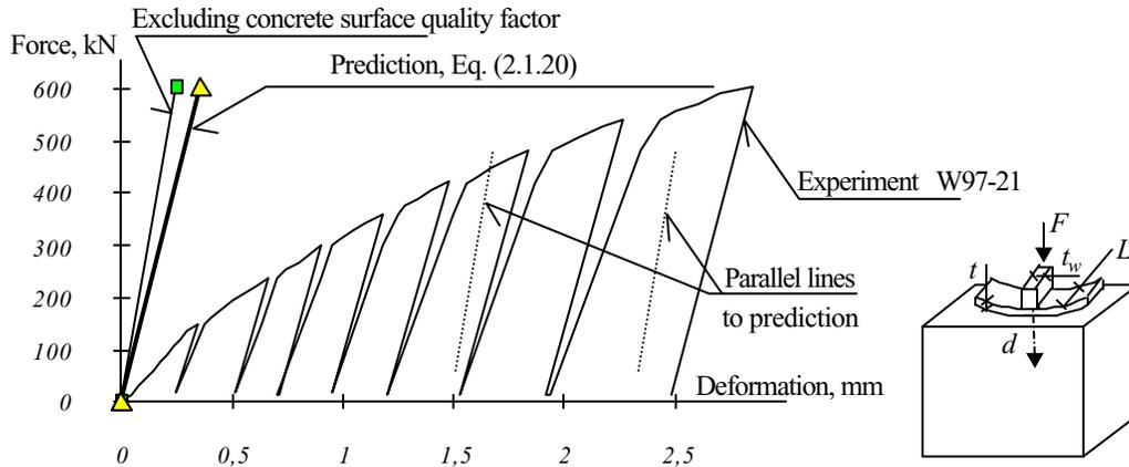
**Figure 2.1.12** Comparison of the stiffness prediction to Test W97-15 repeated and increasing loading, cleaned concrete surface low quality grout (Sokol and Wald, 1997), concrete block  $550 \times 550 \times 500 \text{ mm}$ , plate thickness  $t = 12 \text{ mm}$ , T stub length  $L = 335 \text{ mm}$
