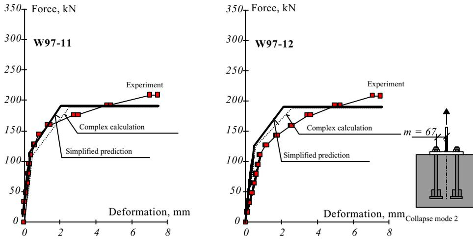
**Figure 2.3.27** Load-deflection diagrams for experiments W 97-11 and W 97-12. (Sokol and Wald, 1997). Bolt M24, plate 20 mm,  $m = 67$  mm,  $n = 40$  mm, concrete block 550 x 550 x 500 mm. Mode 2 collapse (breaking of bolts and plate mechanisms).
