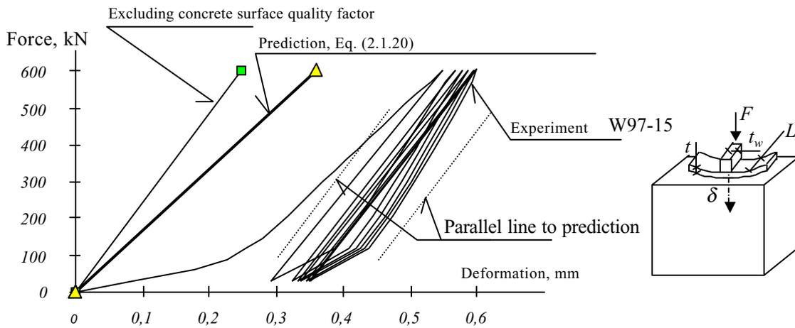
**Figure 2.1.11** Comparison of the stiffness prediction to Test W97-15, repeated loading, cleaned concrete surface without grout only (Sokol and Wald, 1997), concrete block  $550 \times 550 \times 500 \text{ mm}$ , plate thickness  $t = 12 \text{ mm}$ , T stub length  $L = 335 \text{ mm}$
