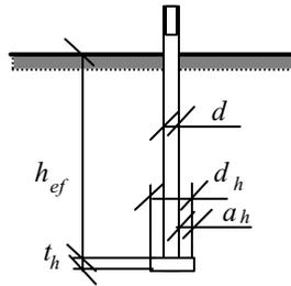
**Figure 2.3.16** Headed embedded anchor bolt
