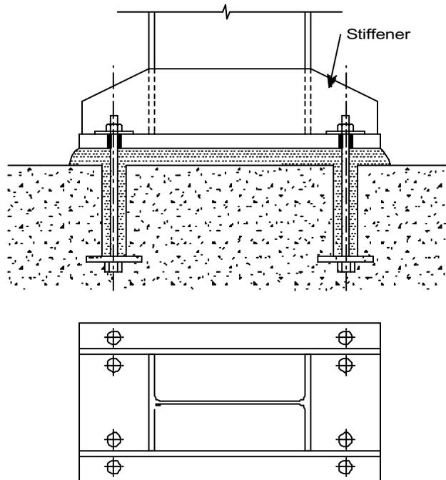
**Figure 1.5** Typical stiffened column base detail
