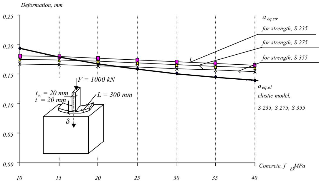
**Figure 2.1.6** Comparison of the prediction of the effective width on concrete - deformation diagram for particular example for unlimited concrete block  $k_j = 5$ , base plate and web thickness  $20 \text{ mm}$ ,  $L = 300 \text{ mm}$ , force  $F = 1000 \text{ kN}$
