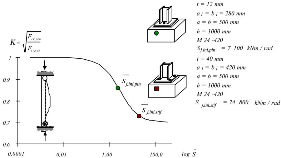
**Figure 5.1** Elastic critical buckling load versus column base initial stiffness
