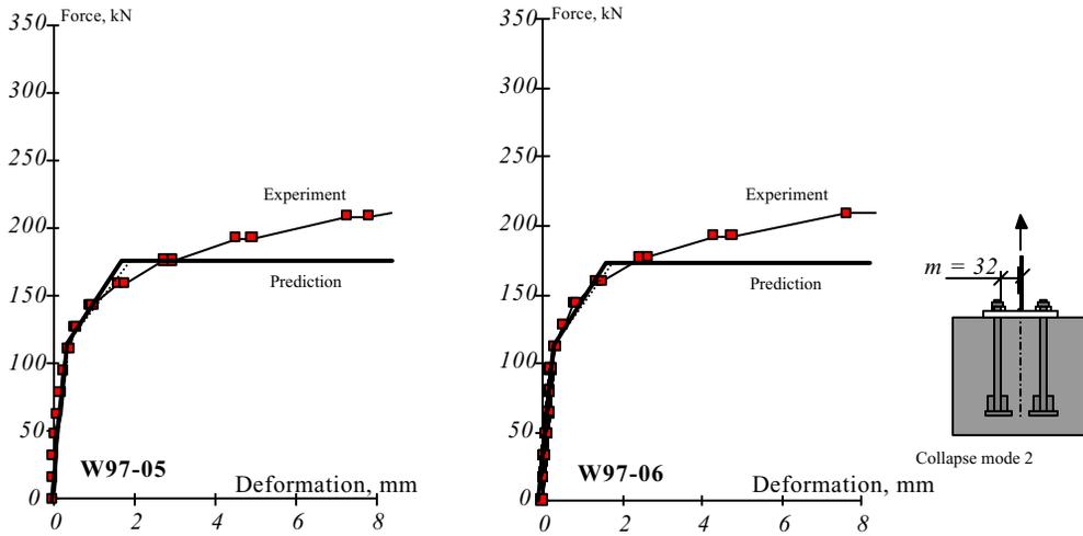
**Figure 2.3.26** Load-deflection diagrams for experiments W 97-05 and W 97-06. (Sokol and Wald, 1997). Bolts M24, plate 12 mm,  $m = 32$  mm,  $n = 40$  mm, concrete block 550 x 550 x 500 mm. Mode 2 collapse (breaking of bolts and plate mechanism).
