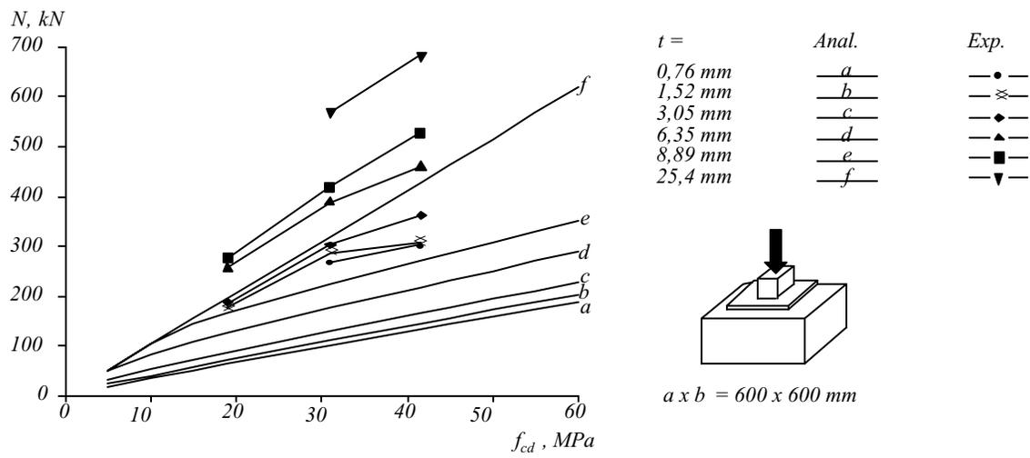
**Figure 2.1.8** Concrete strength - ultimate load capacity relationship (Hawkins, 1968)
