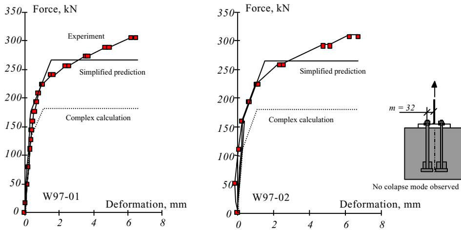
**Figure 2.3.24** Load- deflection diagrams for experiments W 97-01 and W 97-02 (Sokol and Wald, 1997). Bolts M24, plate 20 mm,  $m=32$  mm,  $n=40$  mm, concrete block  $550 \times 550 \times 500$  mm. No collapse was reached due to loading cell limitation
