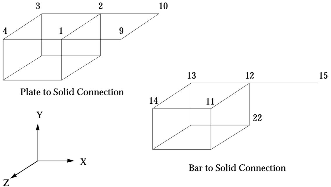
**Figure 19 Transitions Between Element Types**
