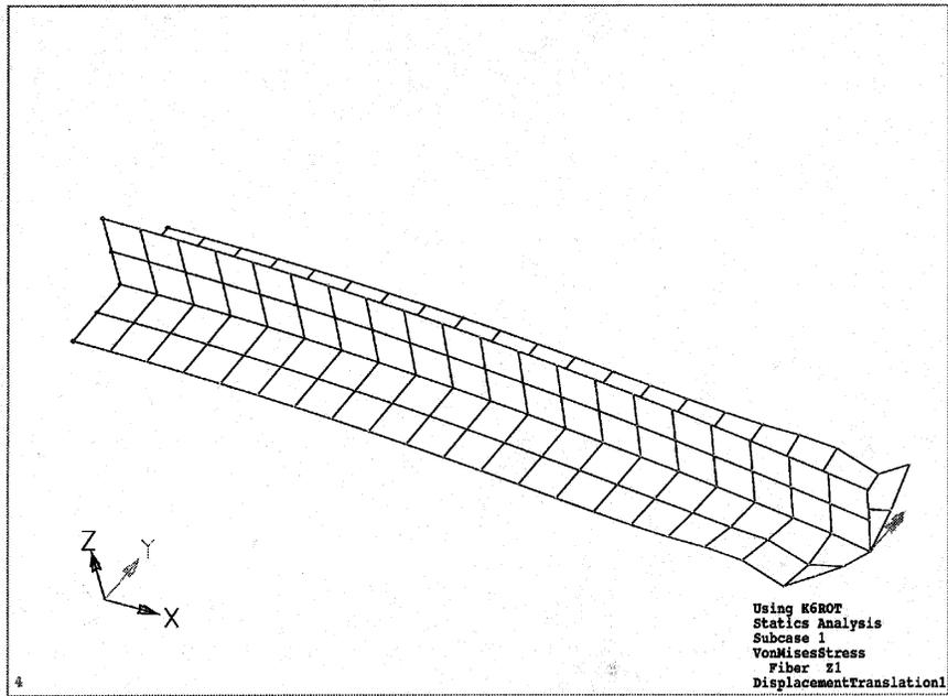
Figure 26 Deformed Shape for Stiffener Modeled with Plate Elements and PARAM, K6ROT
