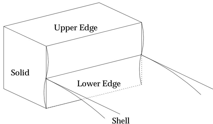
**Figure 20 Clamped Connection of a Shell to a Solid**
