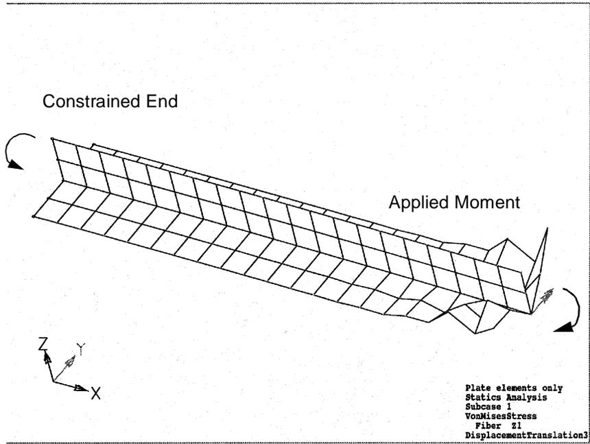
Figure 25 Deformed Shape for Stiffener Modeled with Plate Elements Only
