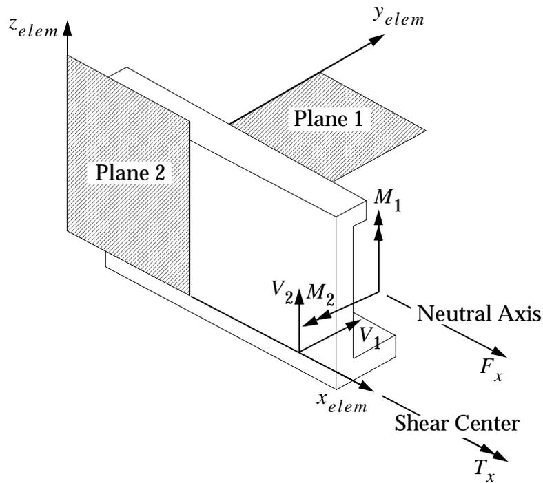
Figure 10 CBEAM Element Forces
