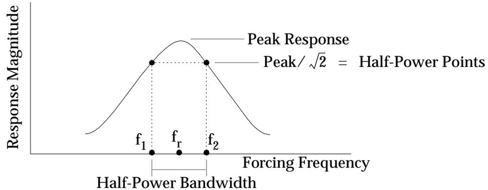
**Figure 44 Half-Power Band Curve**
