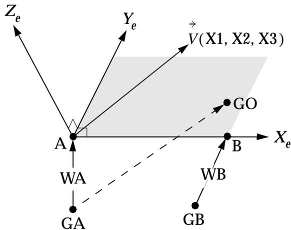
Note that the origin of  $\vec{v}$  is at offset point A when  $\vec{v}$  is defined by components (X1, X2, X3). The origin of  $\vec{v}$  is at GA when  $\vec{v}$  is defined using GO.
