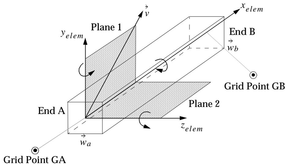
**Figure 5 CBAR Element Coordinate System**
