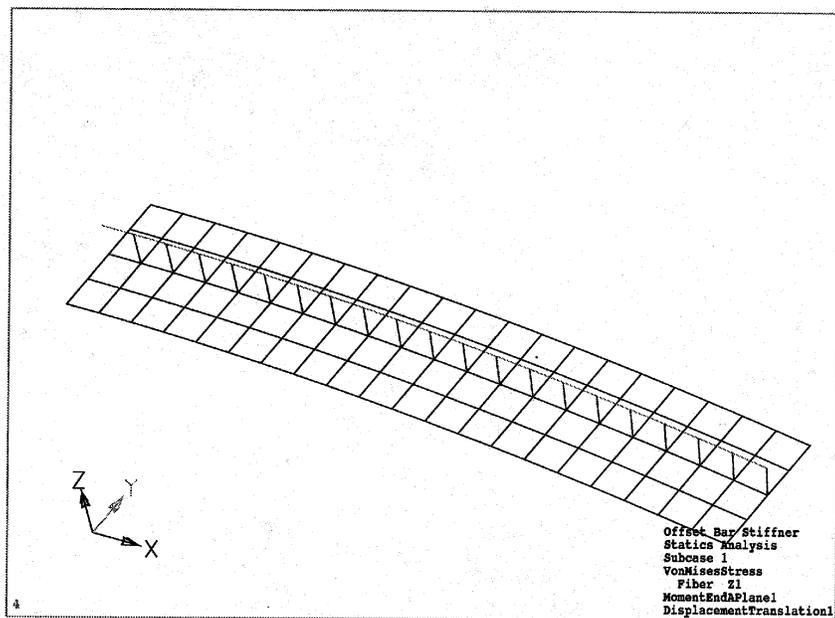
Figure 28 Deformed Shape of Stiffener Modeled with Offset Bar Elements
