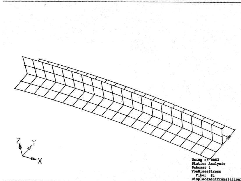
Figure 27 Deformed Shape for Stiffener Modeled with an RBE3 Element at the Tip
