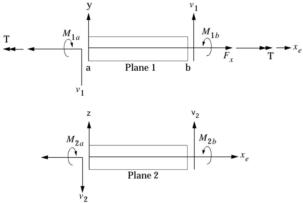
Figure 7 CBAR Element Forces in Plane 1 (top) and Plane 2 (bottom)
