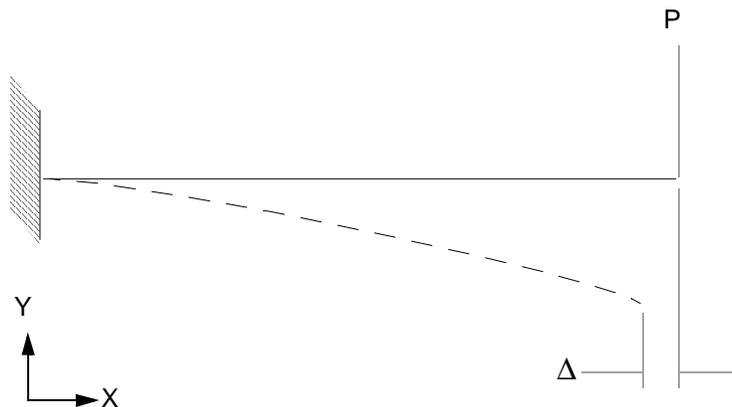
**Figure 24 Cantilever Beam Loaded in the Transverse Direction**
