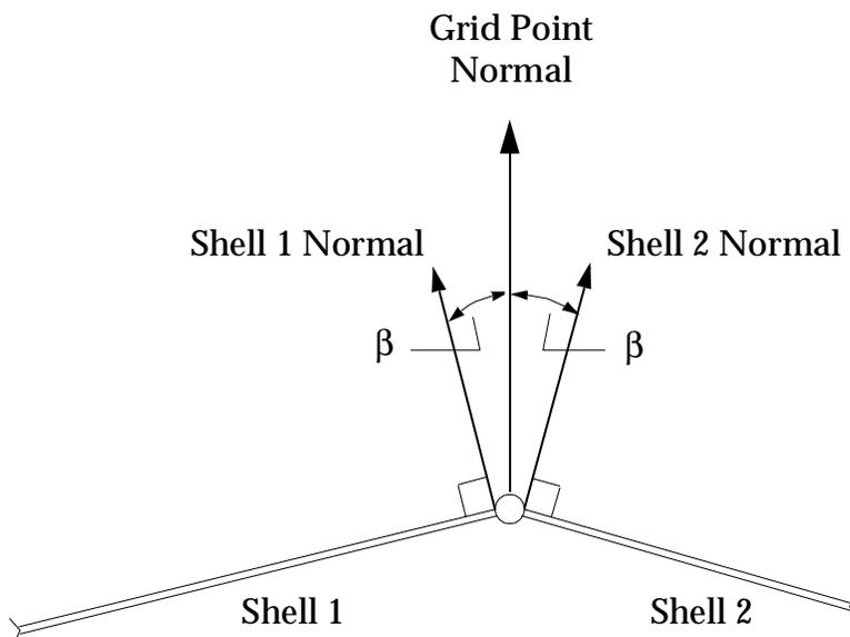
**Figure 12 Unique Grid Point Normal**
