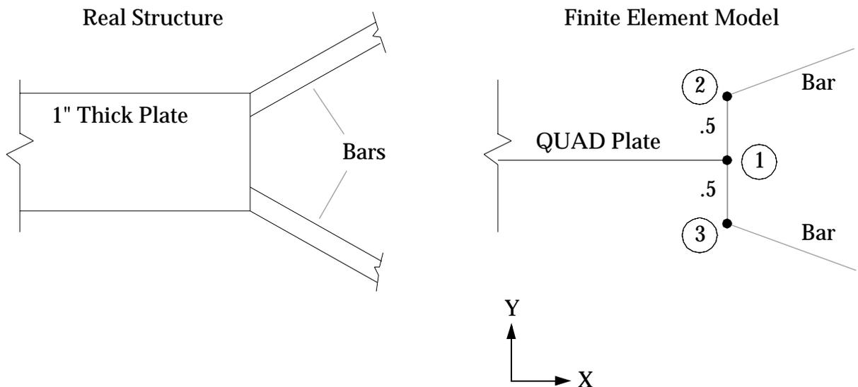
**Figure 15 Model of a Thick Plate with Bars Attached**
