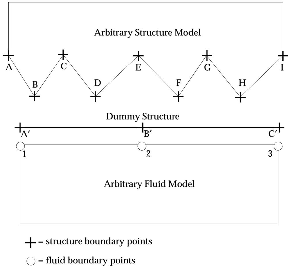
**Figure 29 Non-Coplanar Fluid/Structure Interface**
