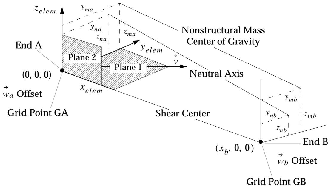
Figure 9 CBEAM Element Coordinate System
