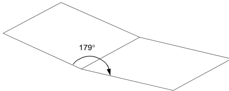
**Figure 11 Two Plates Joined Together That Are Slightly Non-Coplanar**
