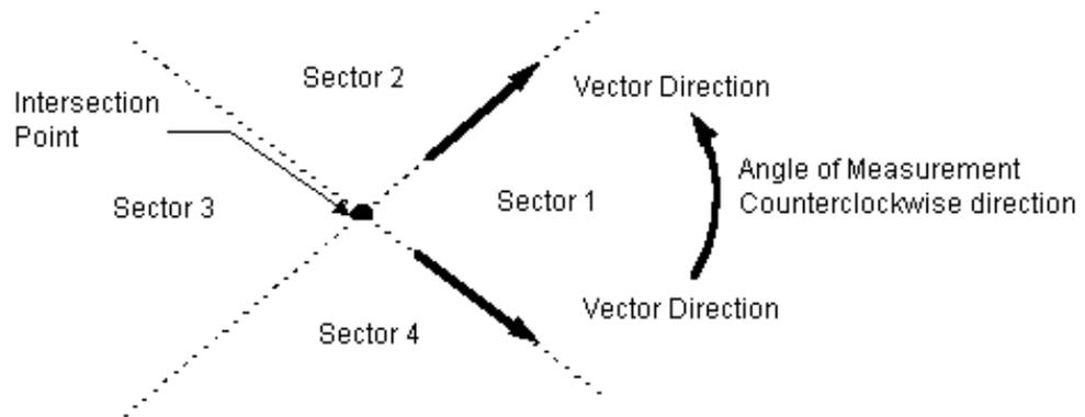
The angles are always measured in the counterclockwise direction with both vector directions going outward from the intersection point (sector one condition). To measure in any other angle, certain properties are set so that the dimension object modifies the vector direction and computes the angle.
