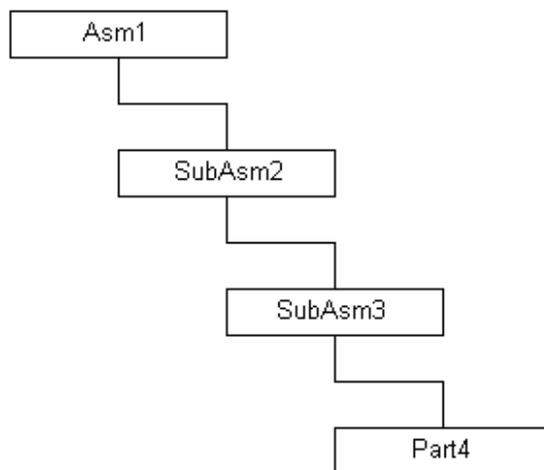
Part4 is a member of SubAsm3, SubAsm3 is a member of SubAsm2, and SubAsm2 is a member of Asm1.
