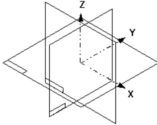
As viewed from a top view, positive x is to the right, positive y is up, and positive z is pointing toward you. The origin of the coordinate system is at the intersection of the three base reference planes as follows:
