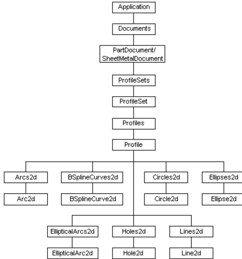
To create a 2-D geometry object, first access a Profile object. The Profile object owns the 2-D graphic object collections, and it is through add methods on these collections that you create geometry. For example, to create a line, you could use the `AddBy2Points` method, which is available through the `Lines2d` collection.
