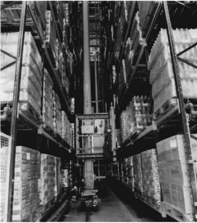
Figure 3.16: Stacker crane, running on a floor-mounted rail.
