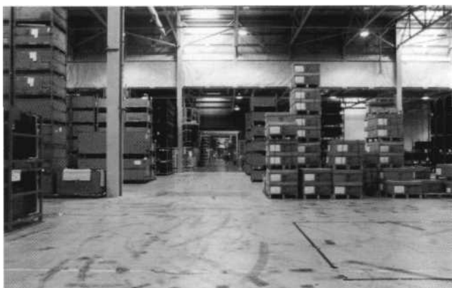
Figure 4.4: A free-movement area: marks from the rubber tyres of the materials handling equipment may be seen.
