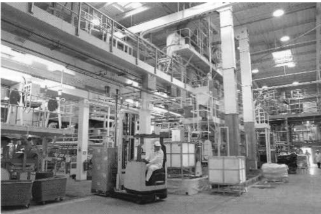
Figure 1.4: The concrete floor in this factory provides a durable platform designed to withstand wear and tear from the materials handling equipment and the products.
