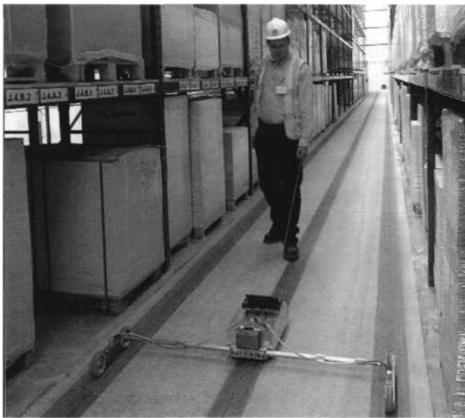
Figure 4.8: Profilegraph in use in an aisle.
