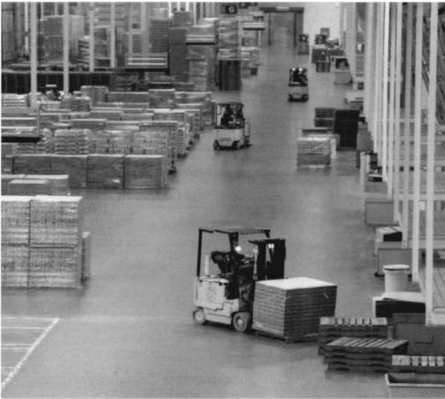
Figure 1.3: A transfer aisle in a large distribution warehouse. Goods are stored in high racking (right) and deposited at the ends of the aisles. Counterbalance trucks then assemble the goods in the collation area for onward distribution.
