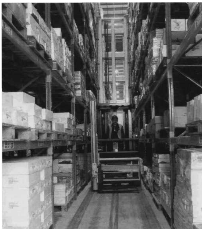
Figure 4.5: A defined-movement area in a very narrow aisle.
