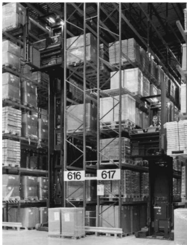
Figure 3.3: Back-to-back storage racking with 'man-up' stacker trucks operating in narrow aisles. Pallets are deposited at the ends of the racking for collection.
