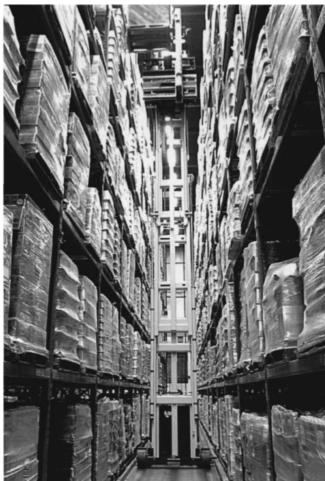
Figure 3.15: 'Man-up' stacker truck in a very narrow aisle warehouse.
