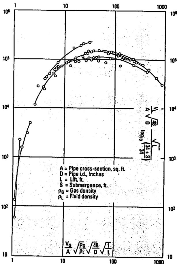
Figure 2. (right) "Correlation" of air-water lift data.
