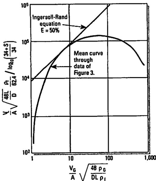
Figure 4. Significance of the Ingersoll-Rand equation.
