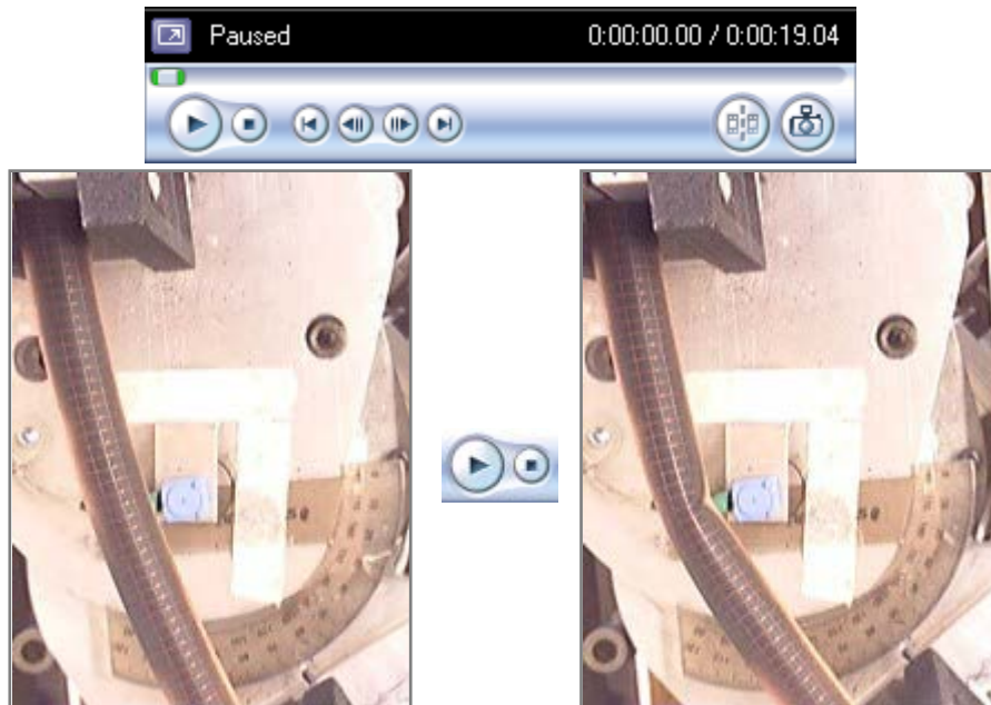
Figure 9: Determining buckling angle with "Play" and "Pause" alone
