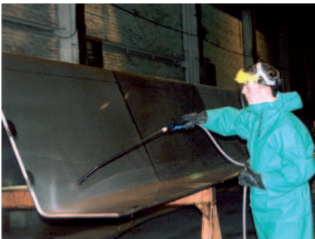
Passivation of what will be part of a chemical tanker bulkhead in duplex stainless steel
