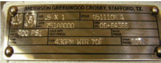
FIGURE 3-12 Typical ASME Section VIII Nameplate
