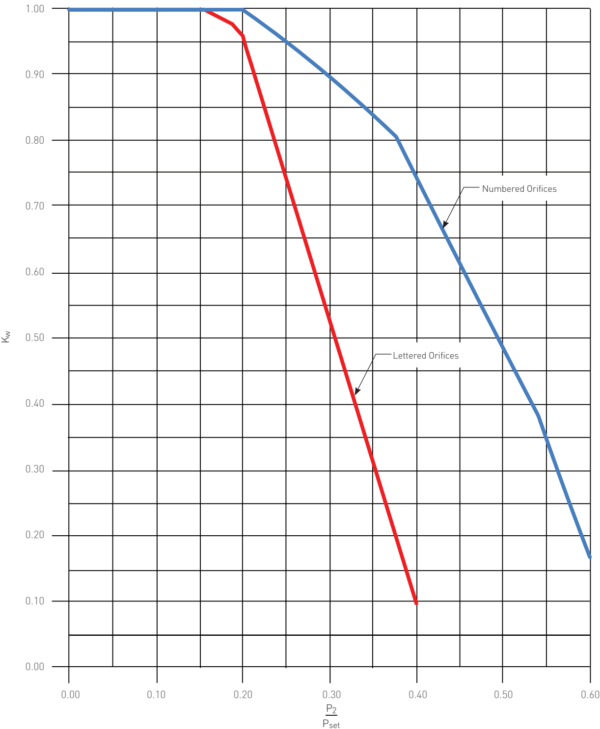
FIGURE 8-19 Anderson Greenwood Series 81P Back Pressure Correction Factor ( K_w ) - Liquid Service
