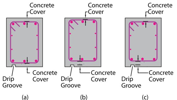
**Fig. 3: Beam sections showing drip groove at bottom soffit: (a) inadequate cover at drip; (b) shifting reinforcing cage to maintain adequate cover at drip will cause top cover problems; and (c) to maintain adequate cover at all locations, stirrup sizes may need to be changed. The designer must consider the effects of shifting or changing the stirrups on beam capacity**
