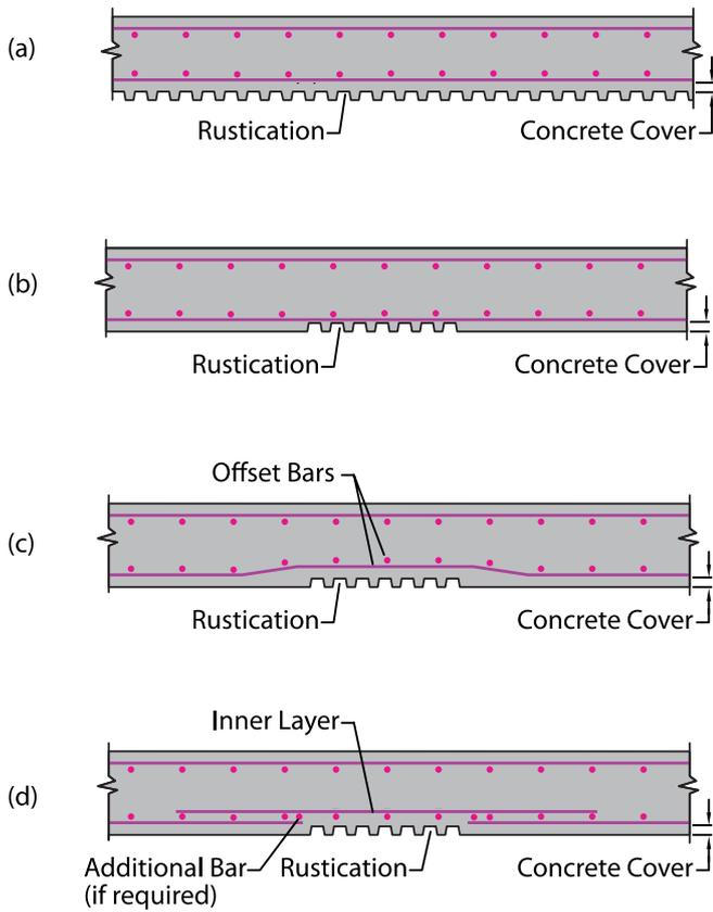
**Fig. 1: Horizontal sections through walls with rustication: (a) rustication considered; (b) rustication not considered; (c) rustication considered using offset bars; and (d) rustication considered using inner layer of bars**
