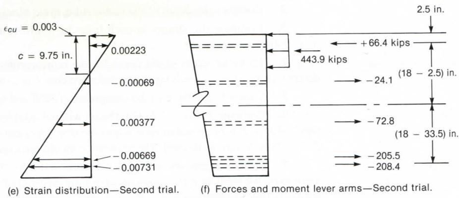
Fig. 5-24 Strain compatibility solution—Example 5-8.
