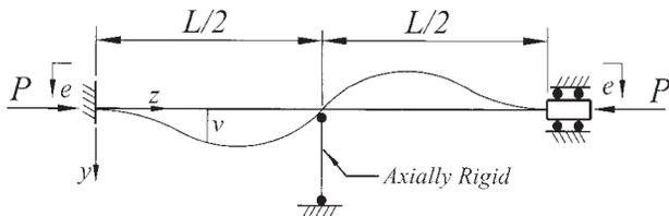
Fig. 6a. Member in axial compression with varying boundary conditions in each plane.
