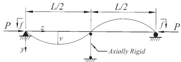
Fig. 7a. Member in axial compression with bracing at mid-point.
