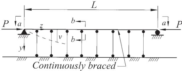
Fig. 1a. Member in axial compression with continuous bracing about one non-principal axis.
