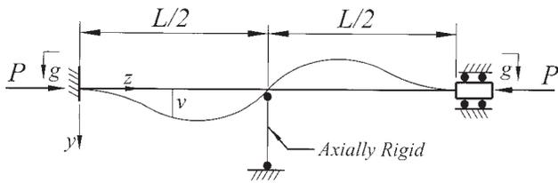
Fig. 8a. Member in axial compression with bracing at mid-point.
