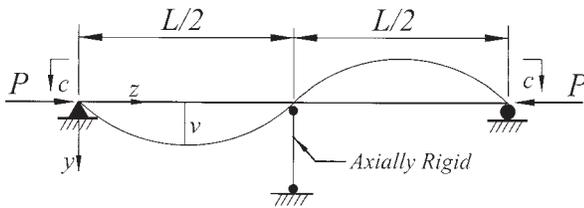
Fig. 4a. Second buckling mode of a simply supported column.
