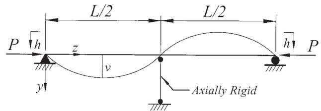
Fig. 9a. Member in axial compression with cross tension member.
