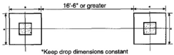
Figure 9-3 Formwork for Drop Panels
