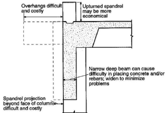
Figure 9-5 Spandrel Beams
