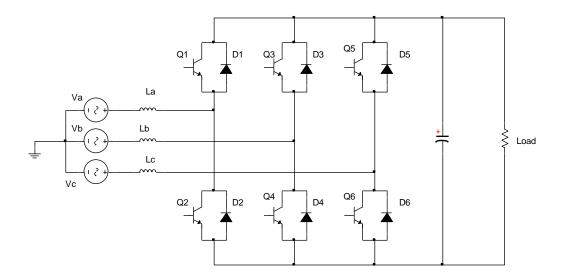
The basic circuit of an IGBT (OK I used a standard NPN transistor – sue me) active rectifier.
