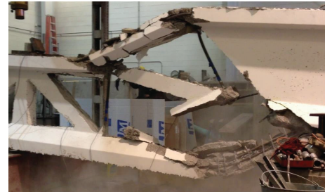
FIGURE 14: Failure of the truss specimen.
