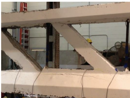
FIGURE 13: Excessive cracking at the bottom flange before failure.
