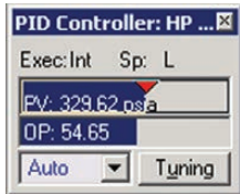
Figure 15: Controller face plate: move the red arrow to adjust the set point, and see how the process variable and controller output respond while the simulation is running
