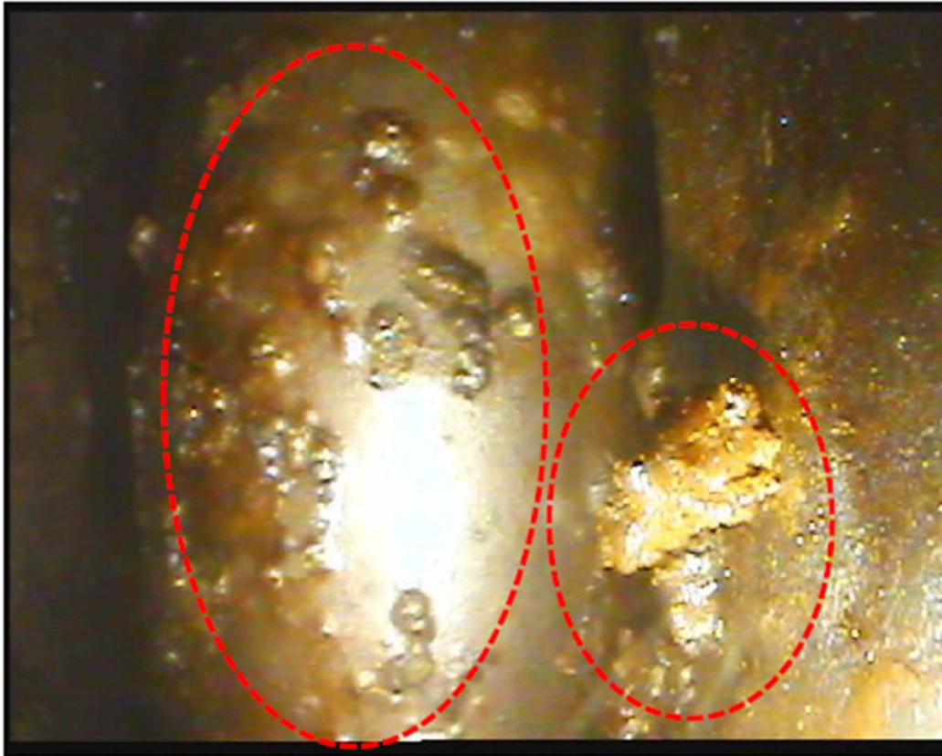
5. Micro Crack (Max. 1.1mm)
