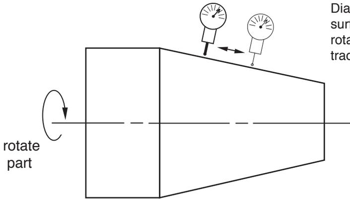
Dial indicator must move along the surface at 15° from the axis of rotation, rather than 0° as in traditional total runout.
