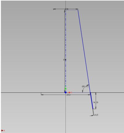
2. Then make coil feature like this: It is important to make a small gap between the coils.
