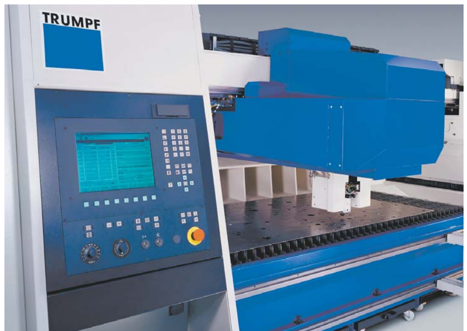
Operator panel in the machine frame.
