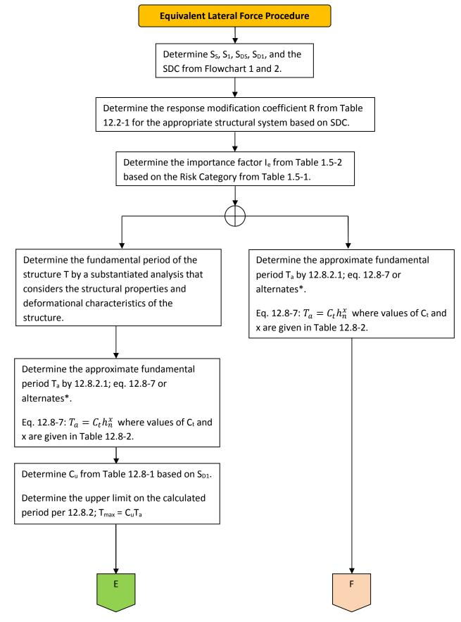
\*Alternative methods for T<sub>a</sub> are given in 12.8.2.1 for concrete and steel moment resisting frames and masonry or concrete shear wall structures.
