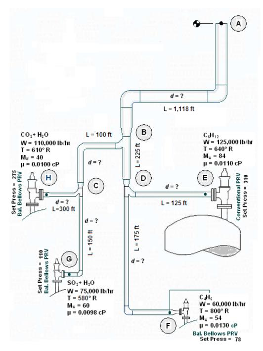
Figure 14a – Relief Discharge Manifold Diagram for Example 12
