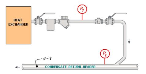
Figure 15 – Relationship between High and Low Pressure Condensate Lines
