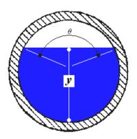
Figure 7 – Relative Flow Depth in Horizontal and Near-Horizontal Pipes
