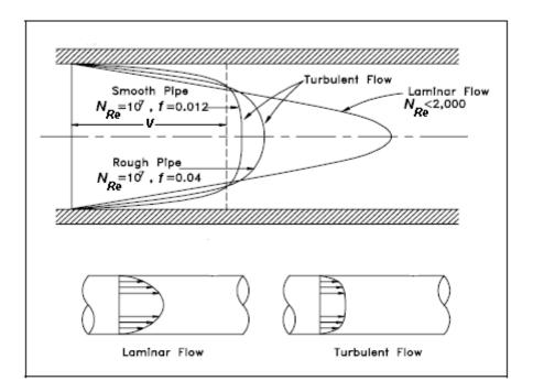
Figure 12 – Velocity Profiles (adapted from Reference 13)
