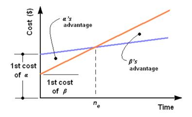
Figure 3 – Break-Even Point of Two Alternative Systems
