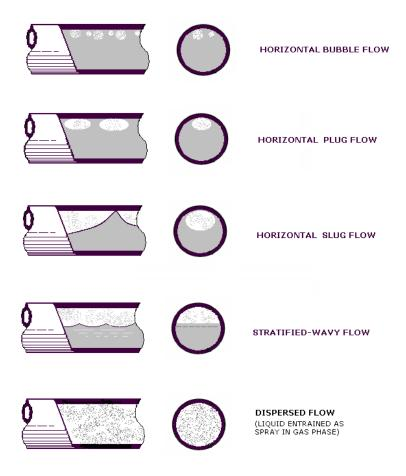
Figure 4 – Flow Patterns in Horizontal Pipes
