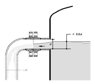
Figure 11 – Static Head to Promote Self-Venting Drainage
