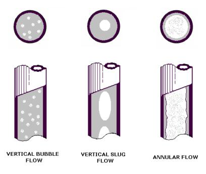
Figure 5 - Flow Patterns in Vertical Pipes
