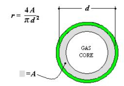
Figure 6 – Plan View of Stack Flow
