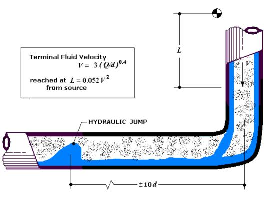
Figure 8 – Vertical to Horizontal Transition Flow
