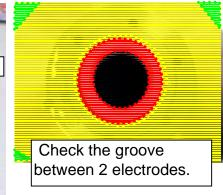
Sensor head has 2 different electrodes, ("Center Electrode" and "Guard Electrode"). These 2 electrodes should be isolated from machine frame, (GND). Furthremore, connector on each side of the cable and BNC relay bracket are not insulated. Check these connectors, make sure they do not to touch GND.
