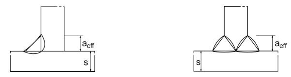
Figure 3.2: Effective weld depth  $a_{\mbox{\scriptsize eff}}$  for shrinkage
