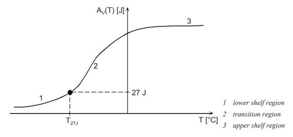
Figure 1.1: Relationship between impact energy and temperature
