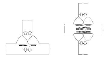
Figure 3.1: Lamellar tearing
