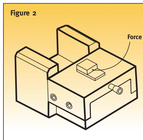
Impact Specimen Fixture with Magnet and
