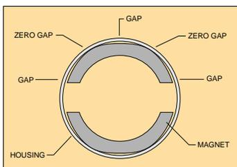
of the tri-arc bond joints shows that the adhesive fixtures or solidifies quickly at the two points of contact on the magnet surface.
