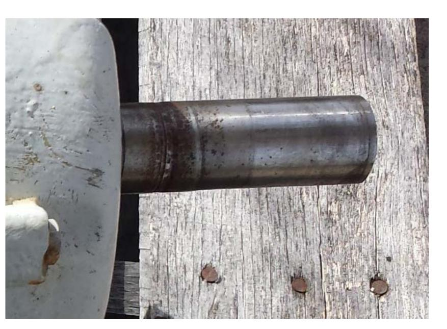
Repaired motor shaft. Machinist repaired the two areas that had grooves in asfound condition by using Speedi-Sleeve. I think these two areas correspond to the lip seals
