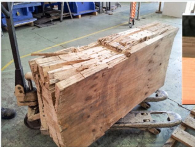
Figure 4: Bearing perpendicular to grain.
