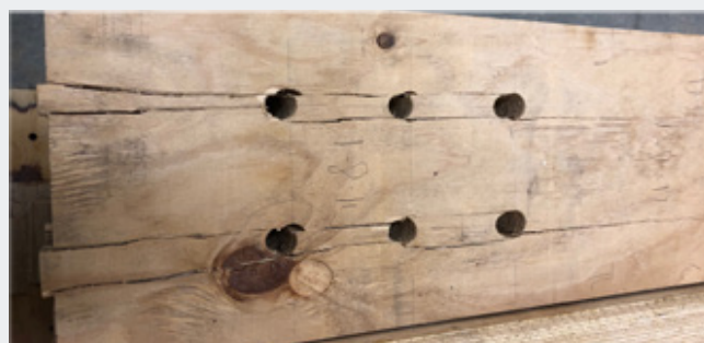
Figure 6: Splitting and row shear failure in connections with multiple large dowel type fasteners.
