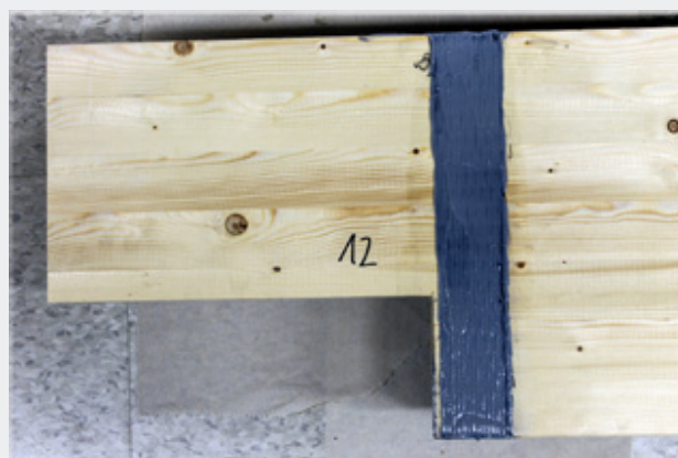
Reinforcement with external Fibre Reinforced Polymer (FRP).
