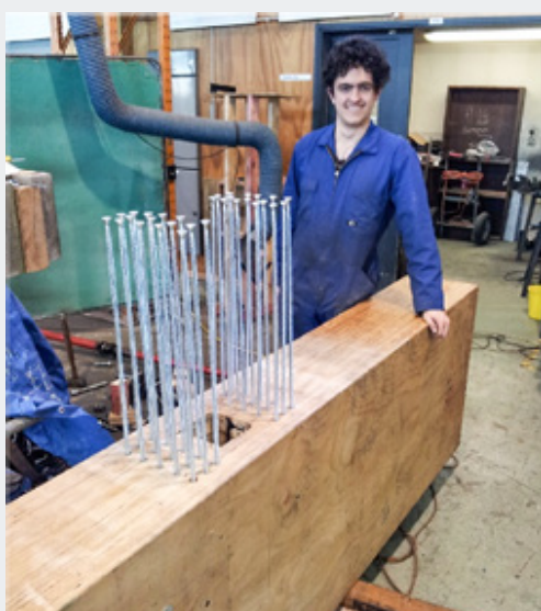
Bearing reinforcement of a Pres-Lam column with fully threaded screws.
