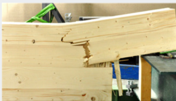
Figure 1: Failure of a notched beam and CLT panel.
