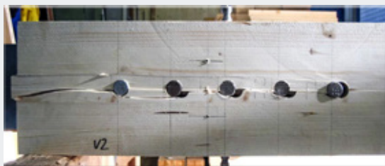
Figure 6: Splitting and row shear failure in connections with multiple large dowel type fasteners.
