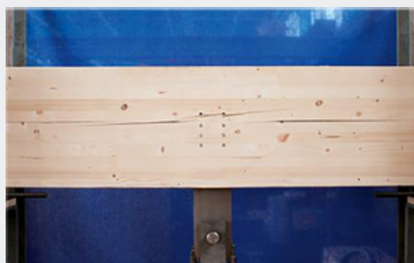
Figure 2: Tension failures at joints loaded perpendicular to grain.
