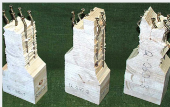
Buckling failure of fully threaded screws embedded in timber (Bejtka, 2005).
