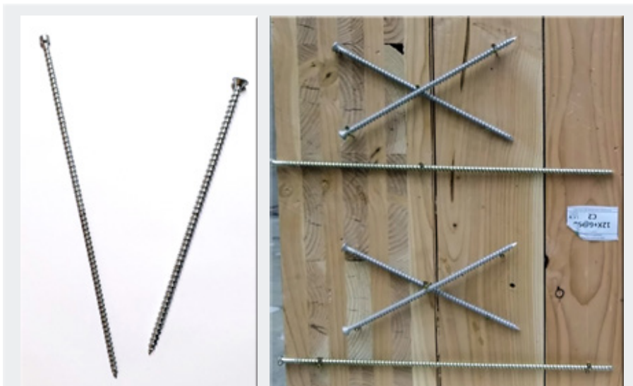
Figure 13: Reinforcement with fully threaded screws.
