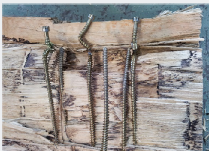
Buckling failure of fully threaded screws embedded in LVL.
