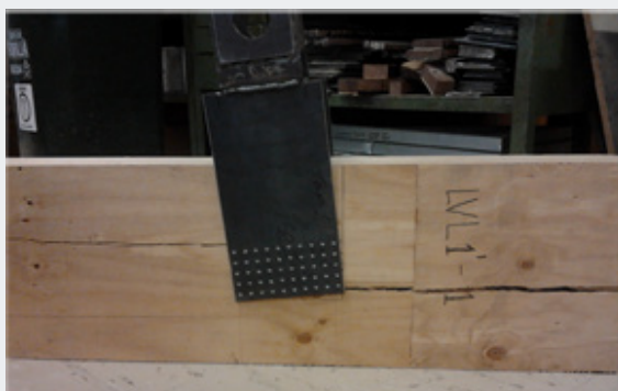
Figure 7: Splitting in moment resisting connections (c/o Pierre Quenneville, University of Auckland and Pouyan Zarnani, Auckland University of Technology).
