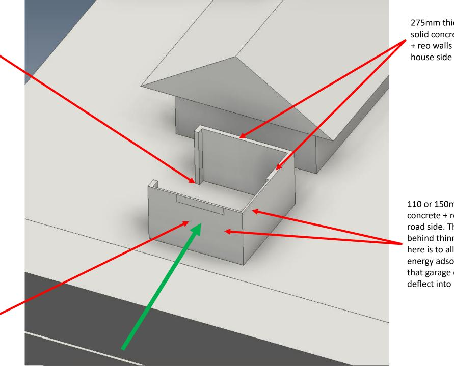
110 or 150mm thick solid concrete + reo walls on road side. The idea behind thinner walls here is to allow for energy adsorption so that garage does not deflect into house
