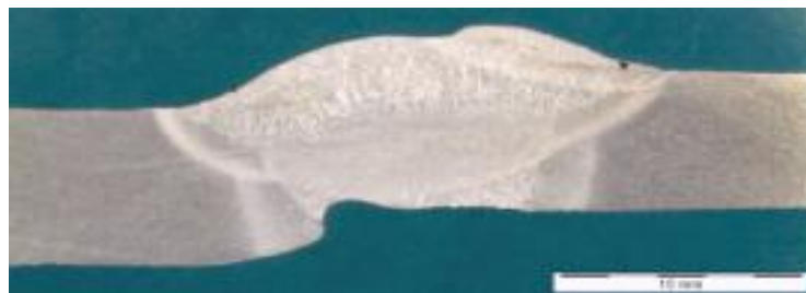
Figure 3. Affected weld with uncentered degradation
