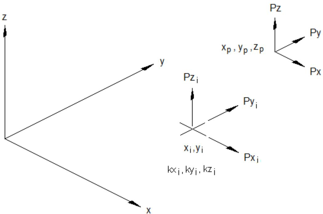
Fastener positions are defined by x and y coordinates ( $x_i, y_i$ ). A spring constant is given for each fastener, where  $k_{x_i}$ ,  $k_{y_i}$ , and  $k_{z_i}$  are spring constants in the x, y, and z directions. Spring constants are for fastener joint shear and axial deflections.
