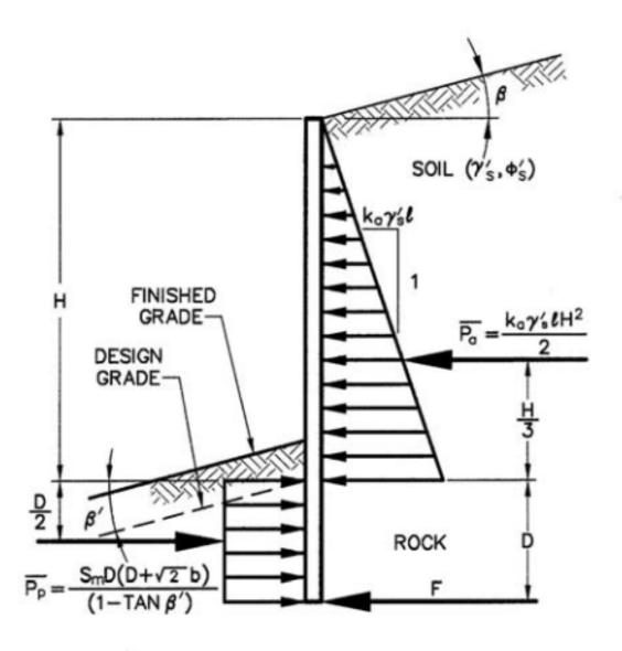
b = ACTUAL WIDTH OF EMBEDDED DISCRETE VERTICAL WALL ELEMENT BELOW DESIGN GRADE IN PLANE OF WALL (FT.).
