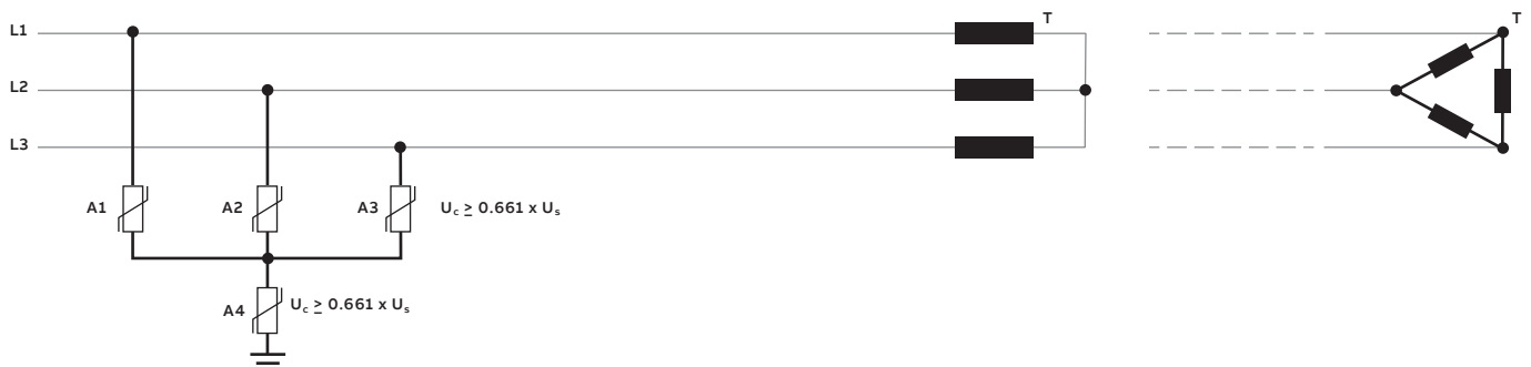
Figure 4: Neptune design with four similar arresters (A1 to A4), each with U_c \geq 0.661 \times U_s .
