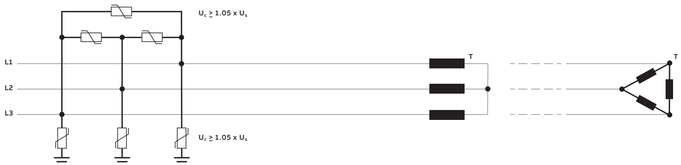
Figure 2: Six-arrester arrangement. All six arresters have the same continuous operating voltage U_c .
