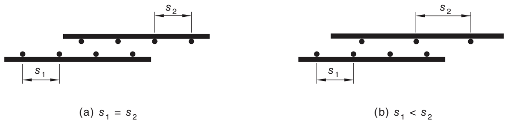
FIGURE 13.2.3 LAPPED SPLICES FOR WELDED MESH
