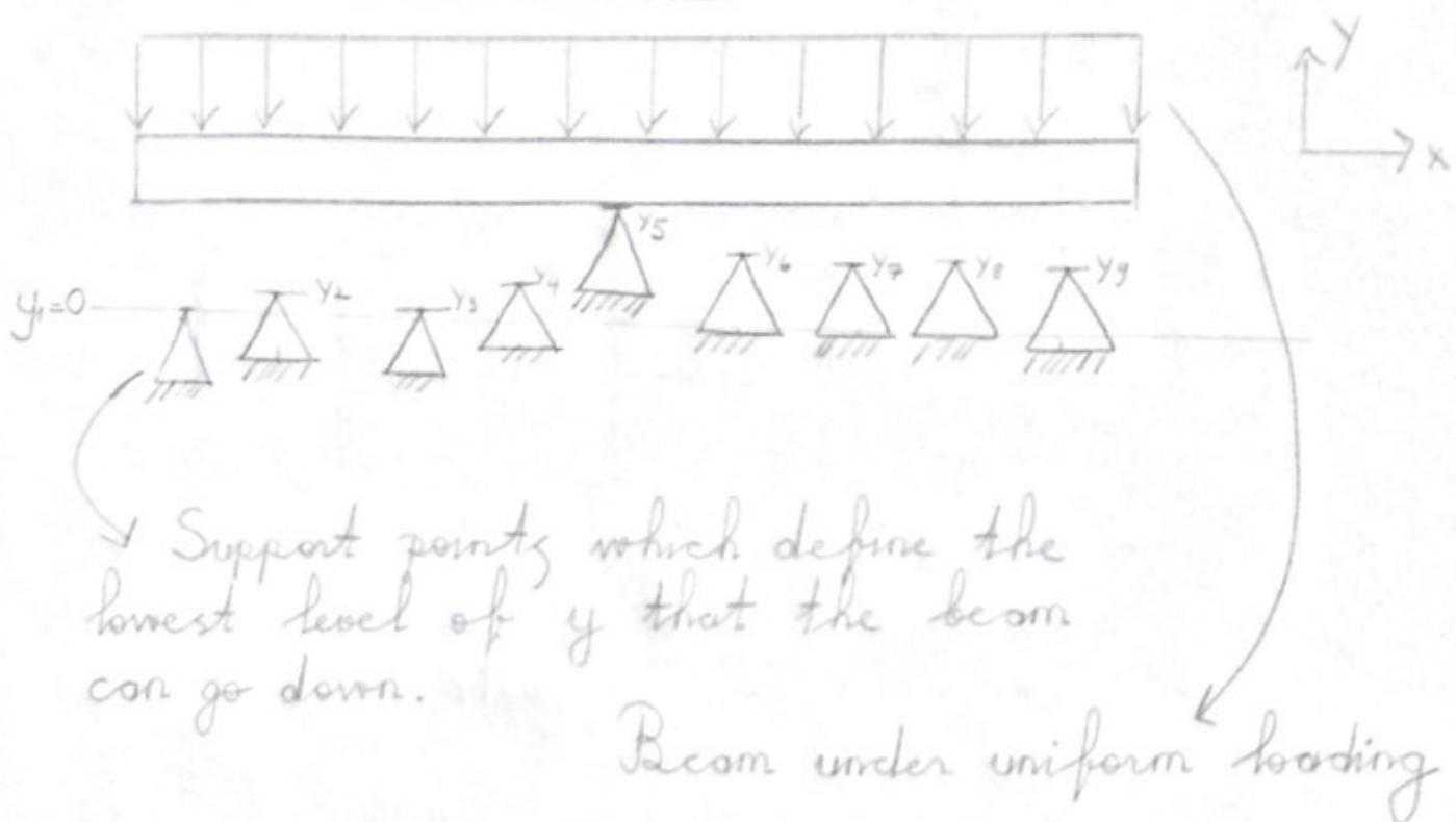
Support points which define the lowest level of  $y$  that the beam can go down.
