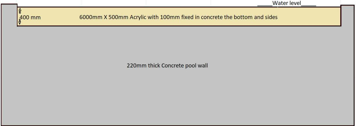
The 500mm Acrylic will be at the top of the pool with water flowing over it into the drain.
