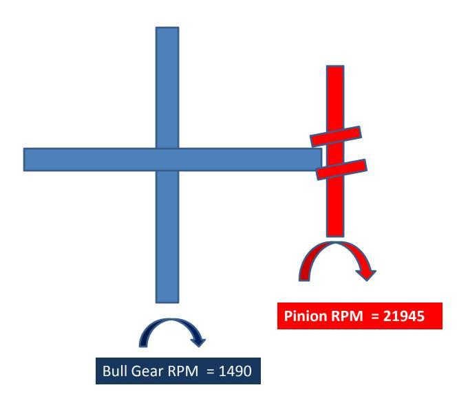
Perfect Pinion Thrust Collar running against perfect Bull Gear having Face Run out (due to position of shaft within Bearings or due to run out on Gear Face or combination of both)
