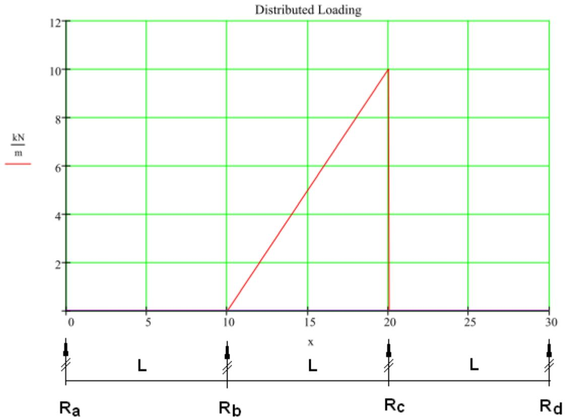
Inputs ...  $E := 200 \cdot \text{GPa}$      $I := 10^8 \cdot \text{mm}^4$      $L := 10 \cdot \text{m}$      $w := 10 \cdot \frac{\text{kN}}{\text{m}}$
