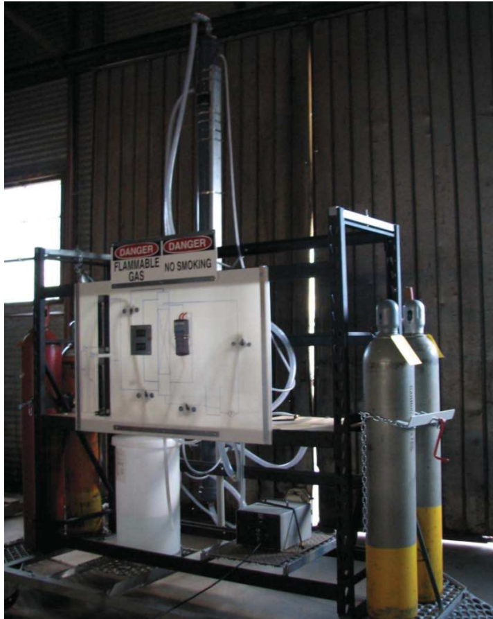
Figure 9.7: Experimental biogas purification set-up.
