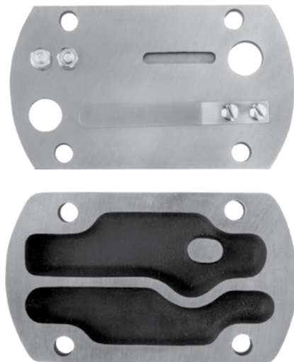
Figure 2.34 A reed valve showing the reed (upper view) and the air or gas passages, (lower view).
