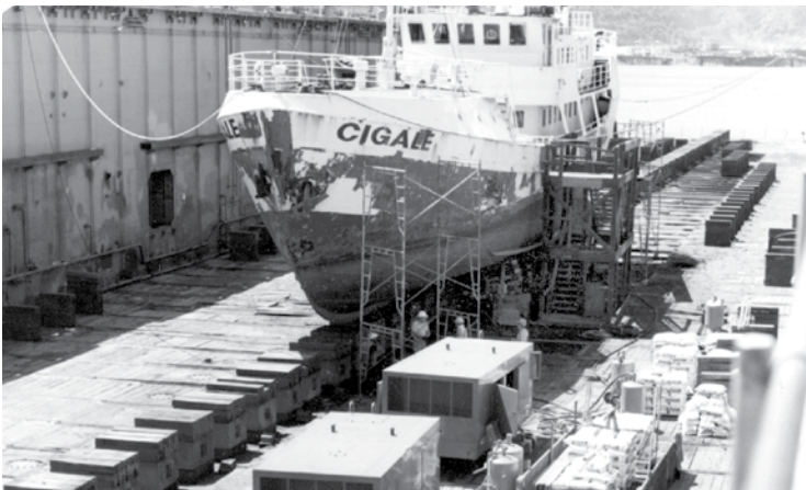
Figure 2.22 Two portable compressors being readied for the job of sandblasting a ship in dry dock to remove rust. The housing doors will be closed during the actual work.
