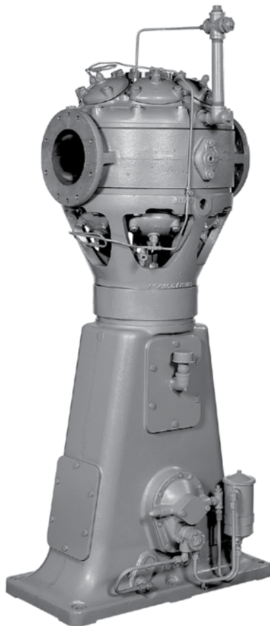
Figure 2.48 A Single Cylinder, Oil Free, Double-Acting Compressor with Vertical, Single-Throw Frame
