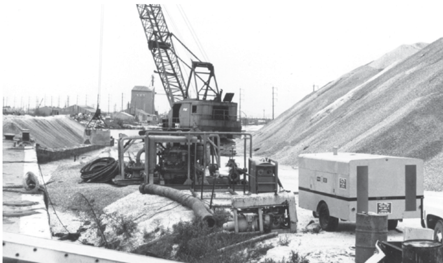
Figure 2.23 A 265 cfm, 125 psig silenced portable air compressor on site at an oyster shell barge.
