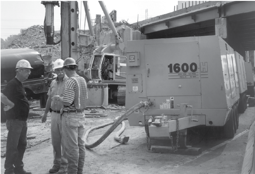
Figure 2.14 Three portable air compressors provide high pressure compressed air for pile driving operations on a U.S. interstate highway project. Each compressor delivers 1600 cfm of air at 150 psig.
