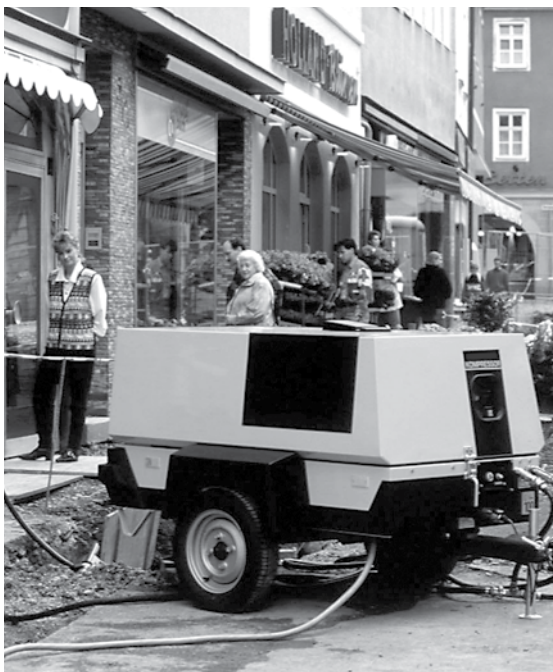
Figure 2.17 A silenced portable compressor in use in a residential area.
