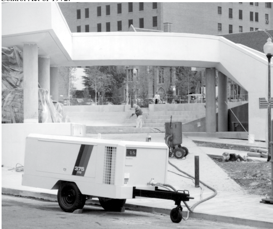
Figure 2.13 Portable compressor with a noise limiting housing suitable for use in residential areas, even near hospitals.
