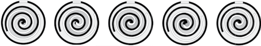
Figure 2.11 Operating Principle for a Scroll Compressor
