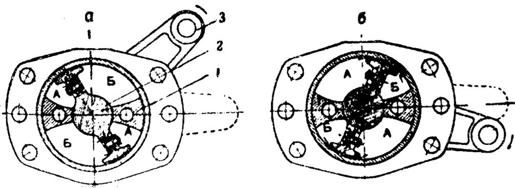
Fig. 165. Working of shock absorber.
