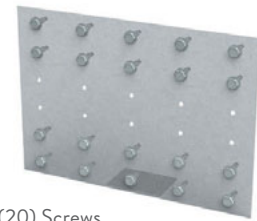
(20) Screws (12) at Header (8) at Jamb
