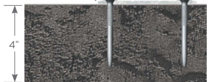
Powder-Actuated Fasteners in Concrete
