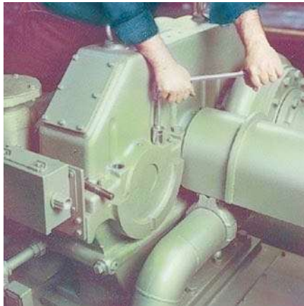
Horizontally split gearbox offers easy access to internal components.
