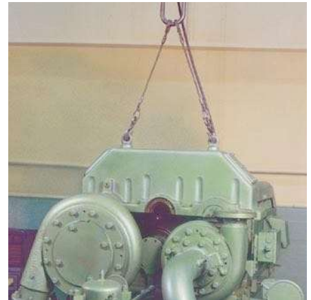
Bearings, gears and seals immediately accessible with gearbox cover removal.
