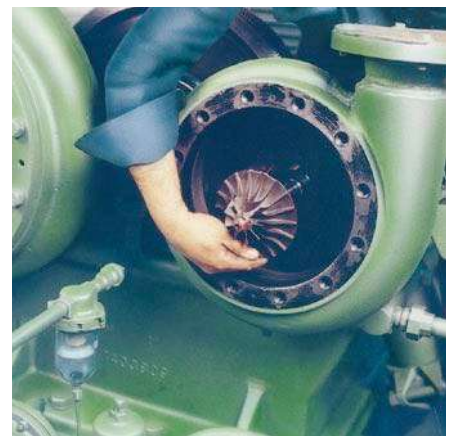
Impeller is revealed for inspection or simple removal.
